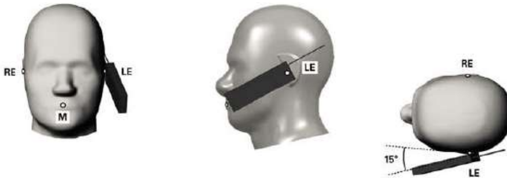
Fig.11.4 Illustration for Tilted Position
