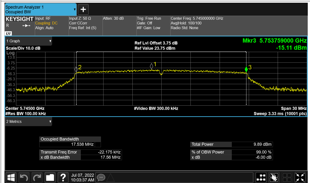
-6dB Bandwidth NVNT n20 5785MHz Ant1
