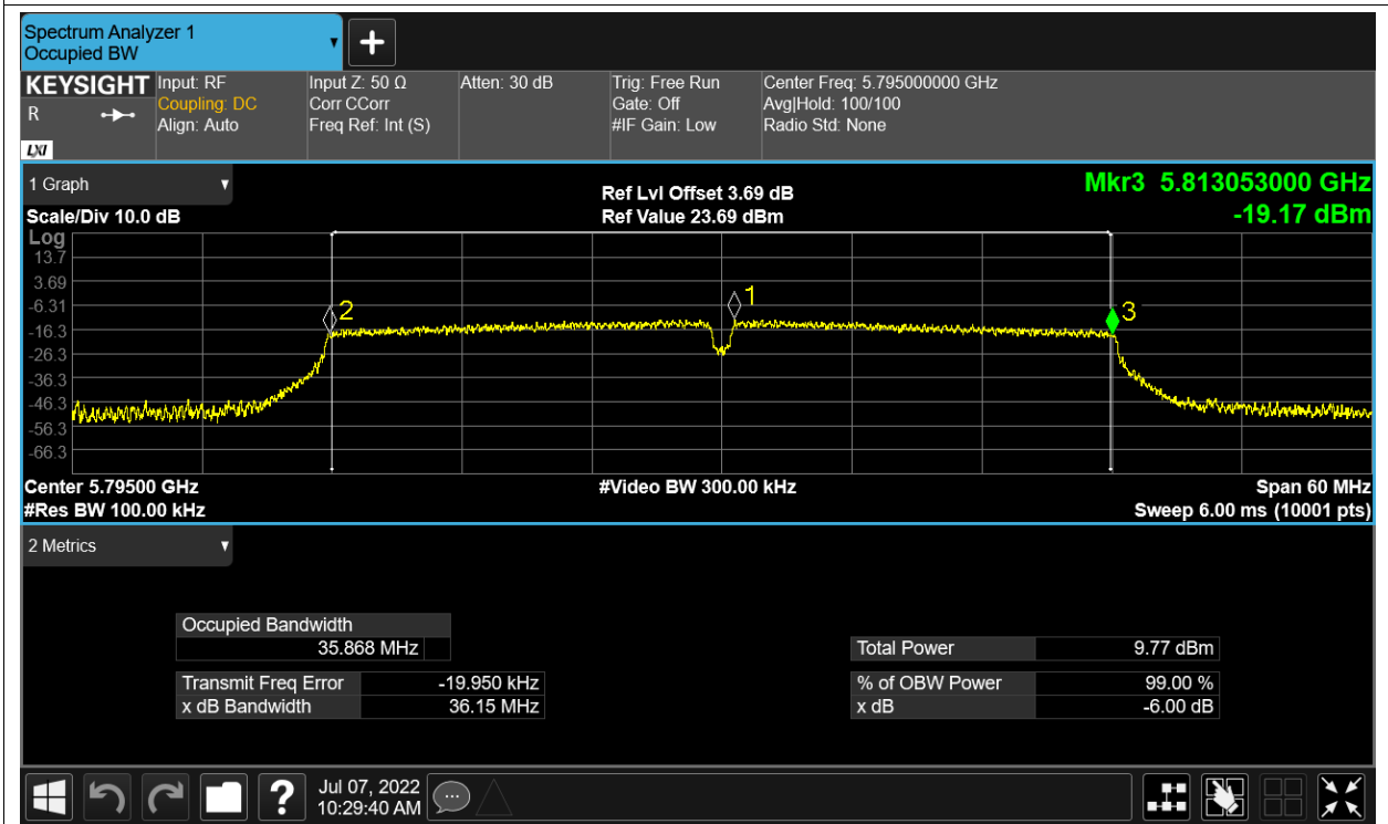
-6dB Bandwidth NVNT ac80 5775MHz Ant1
