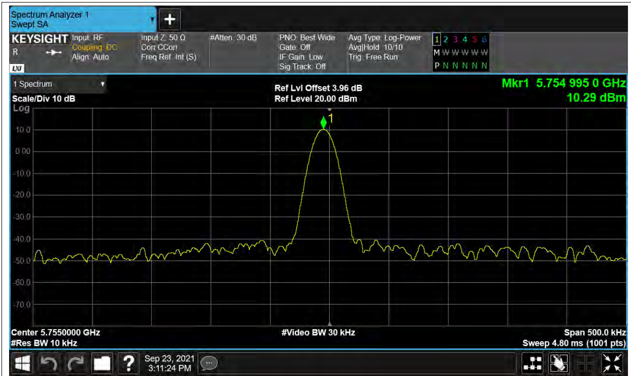
Freq. Stability NVNT ac40 5755MHz MIMO
