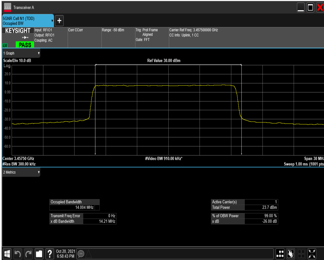
n78(3450-3550) SCS=15kHz DFT_QAM256 BW=15MHz Channel=630500 RB=75@0
