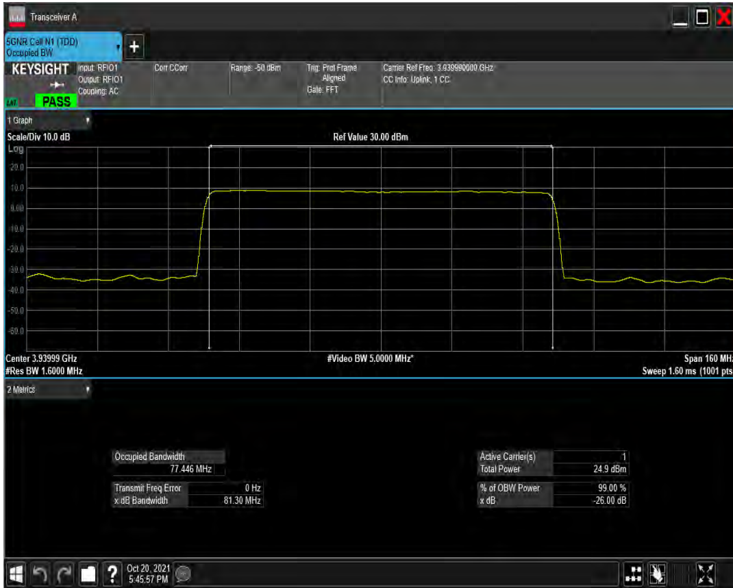
n77(3700-3980) SCS=30kHz DFT_QPSK BW=80MHz Channel=662666 RB=216@0
