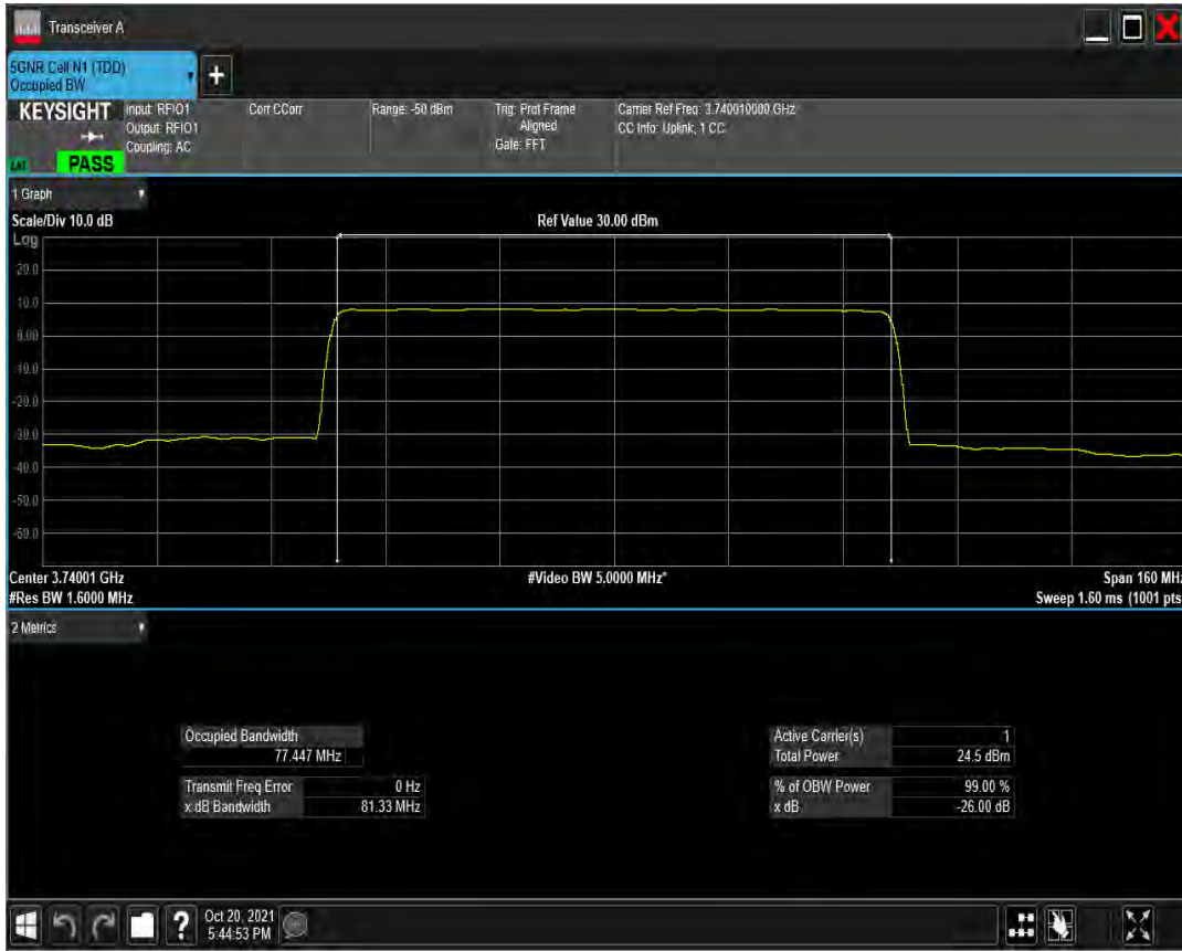
n77(3700-3980) SCS=30kHz DFT_QAM16 BW=80MHz Channel=649334 RB=216@0
