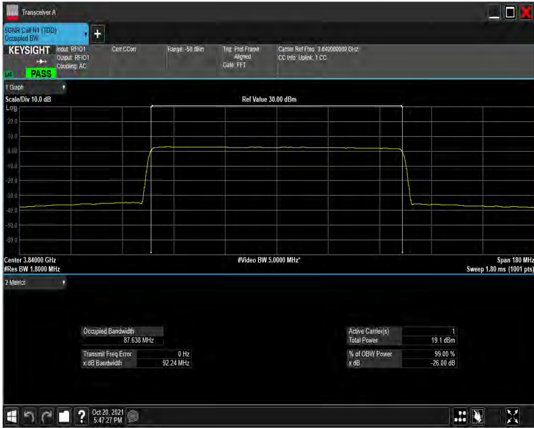
n77(3700-3980) SCS=30kHz DFT_BPSK BW=100MHz Channel=656000 RB=270@0
