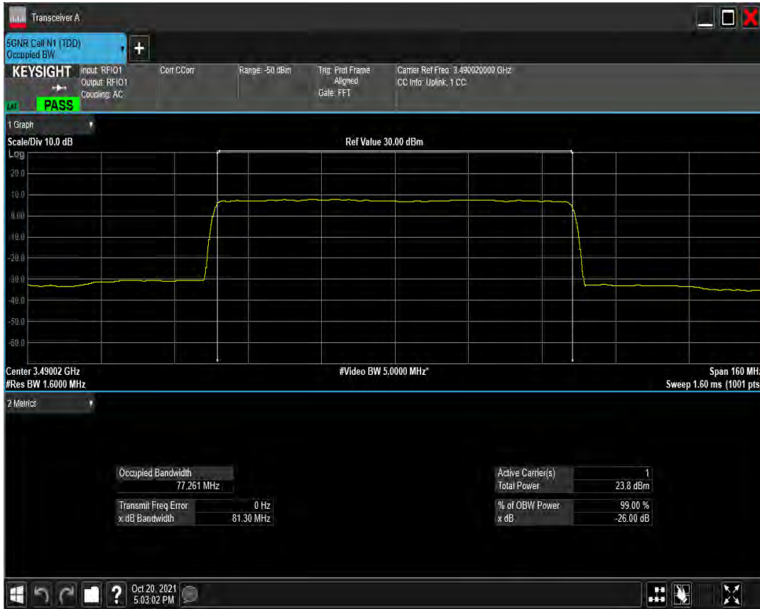
n77(3450-3550) SCS=30kHz DFT_QAM64 BW=80MHz Channel=632668 RB=216@0
