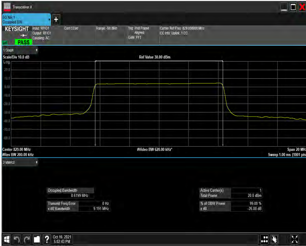
n5 SCS=30kHz CP_QAM16 BW=10MHz Channel=165800 RB=24@0
