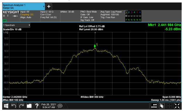
Tx. Spurious NVNT BLE 2442MHz Ant1 Emission
