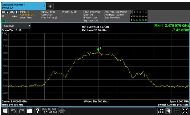
Tx. Spurious NVNT BLE 2480MHz Ant1 Emission
