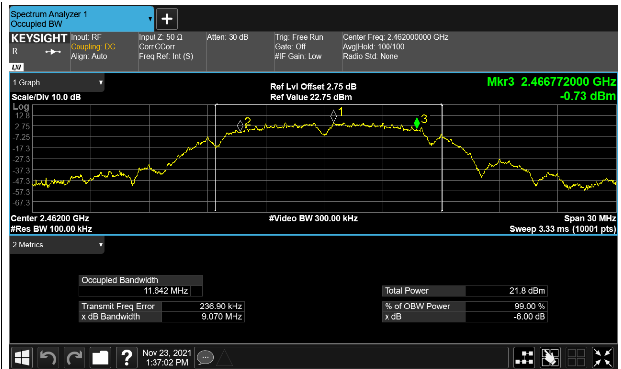
-6dB Bandwidth NVNT g 2412MHz Ant1
