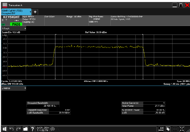
n66_40MHz_15kHz_1745MHz_CP-OFDM 64 QAM_RB216@0 38.466MHz
