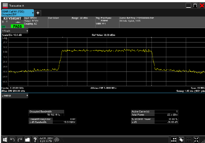
n38_20MHz_30kHz_2595MHz_CP-OFDM 64 QAM_RB51@0 18.162MHz
