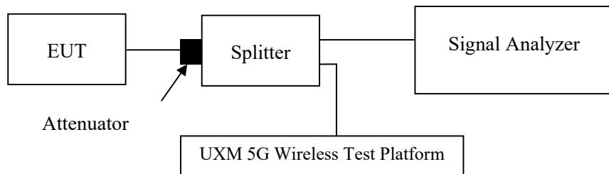
Note: the worst path loss (cable loss and splitter inset loss) among the test frequency range was added into plots.
