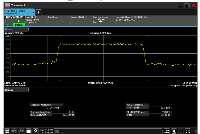
n78_3_40MHz_30kHz_3750MHz_DFT-s-OFDM 16 QAM_RB100@0 37.286MHz
