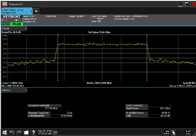
n78_3_40MHz_30kHz_3720MHz_CP-OFDM 256 QAM_RB106@0 37.781MHz
