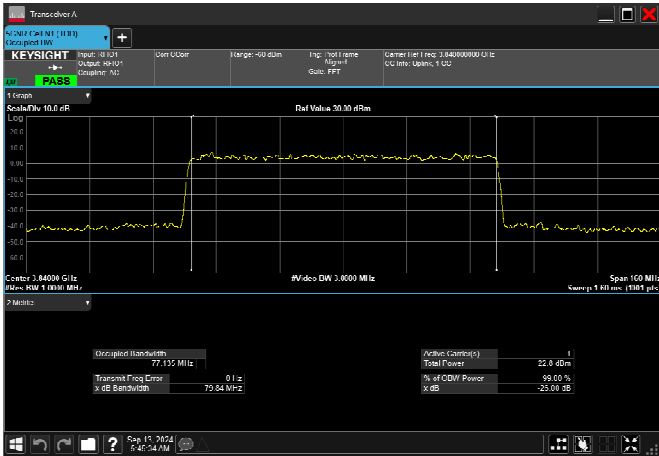
n77_3_80MHz_30kHz_3840MHz_CP-OFDM QPSK_RB217@0 77.451MHz
