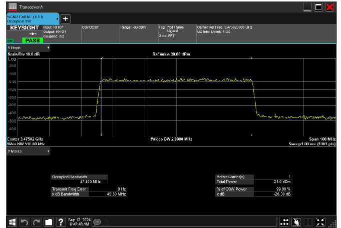
n77_1_50MHz_30kHz_3500MHz_DFT-s-OFDM \pi/2 BPSK_RB128@0 47.039MHz
