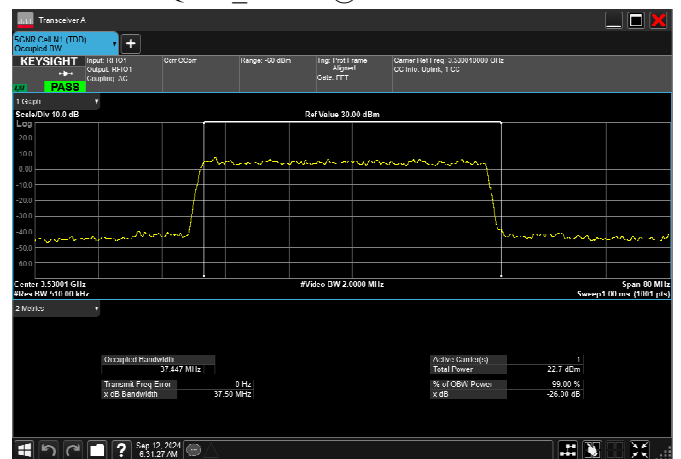
n77_1_40MHz_30kHz_3530MHz_DFT-s-OFDM 16 QAM_RB100@0 37.447MHz
