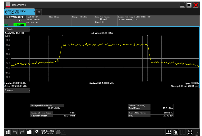
n78_1_20MHz_30kHz_3500MHz_CP-OFDM 256 QAM_RB51@0 18.183MHz
