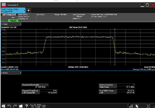
n78_1_30MHz_30kHz_3500MHz_DFT-s-OFDM 256 QAM_RB75@0 27.505MHz
