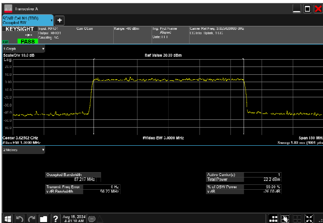
n77_2_90MHz_30kHz_3625MHz_CP-OFDM 64 QAM_RB245@0 87.217MHz
