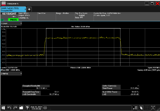
n77_2_100MHz_30kHz_3625MHz_DFT-s-OFDM 16 QAM_RB270@0 96.447MHz
