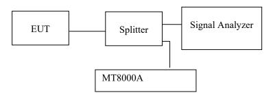
Note: the worst case path loss (cable loss and splitter inset loss) among the test frequency range has included in plots.
