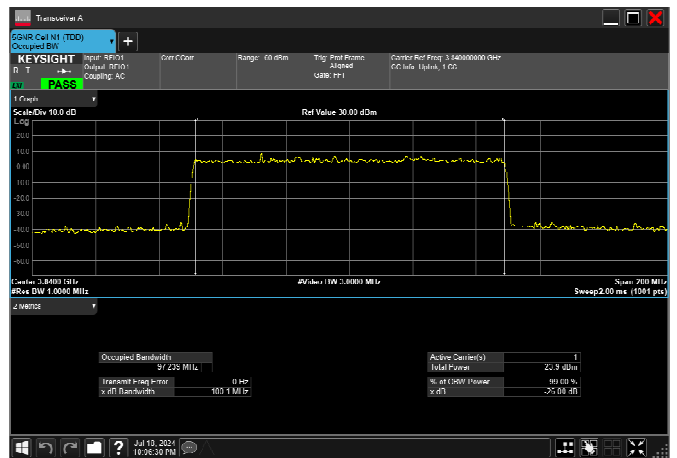
n77_3_100MHz_30kHz_3840MHz_CP-OFDM 256 QAM_RB273@0 97.239MHz
