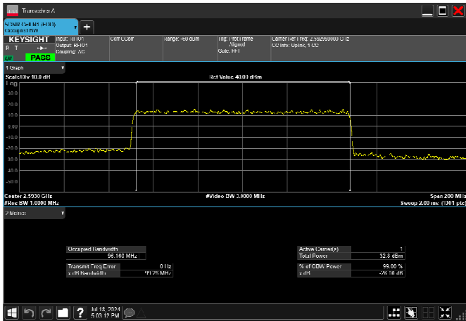
n41_100MHz_30kHz_2592.99MHz_DFT-s-OFDM 256 QAM_RB270@0 96.443MHz
