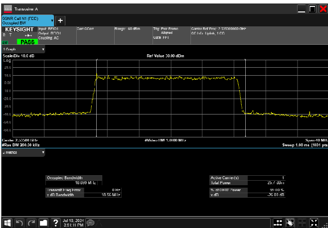
n7_20MHz_15kHz_2535MHz_DFT-s-OFDM QPSK_RB100@0 18.899MHz
