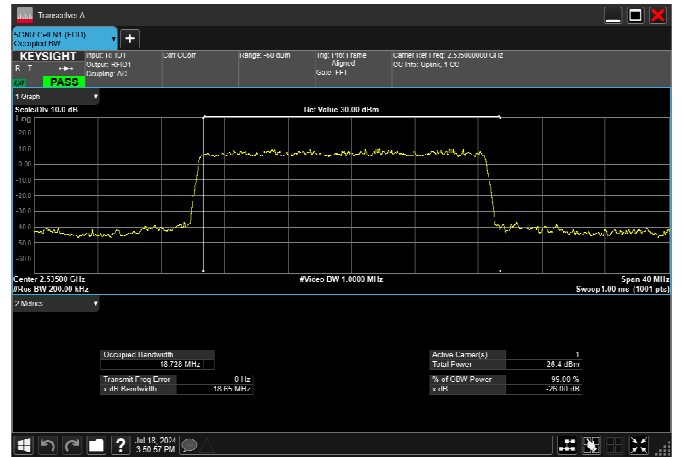
n7_20MHz_15kHz_2535MHz_DFT-s-OFDM 16 QAM_RB100@0 18.675MHz
