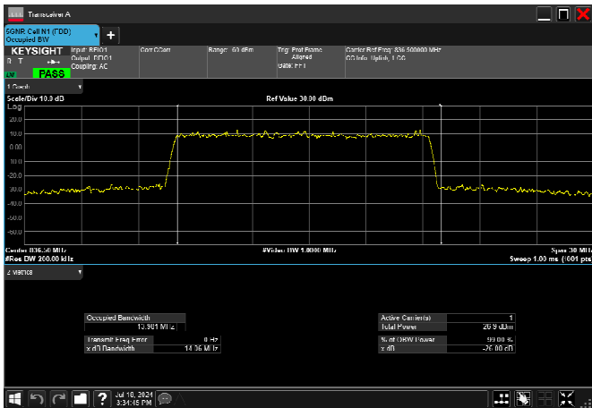
n5_15MHz_15kHz_836.5MHz_DFT-s-OFDM 256 QAM_RB75@0 13.981MHz
