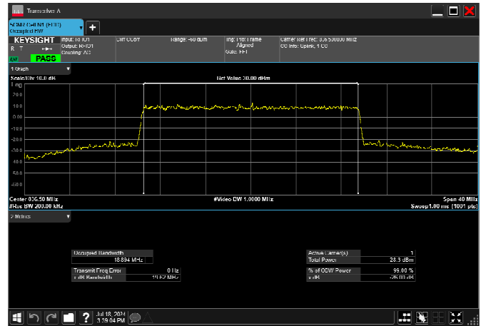
n5_20MHz_15kHz_836.5MHz_CP-OFDM 256 QAM_RB106@0 18.900MHz
