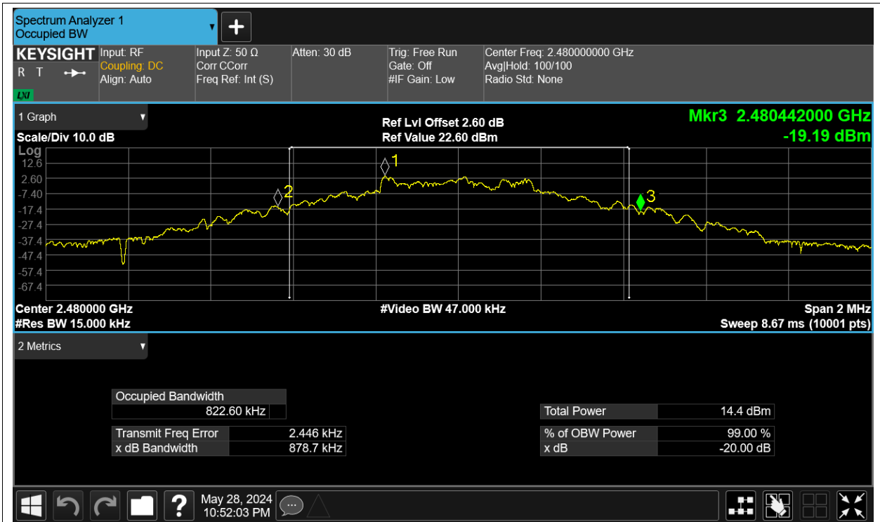
-20dB Bandwidth NVNT 2-DH1 2402MHz Ant1
