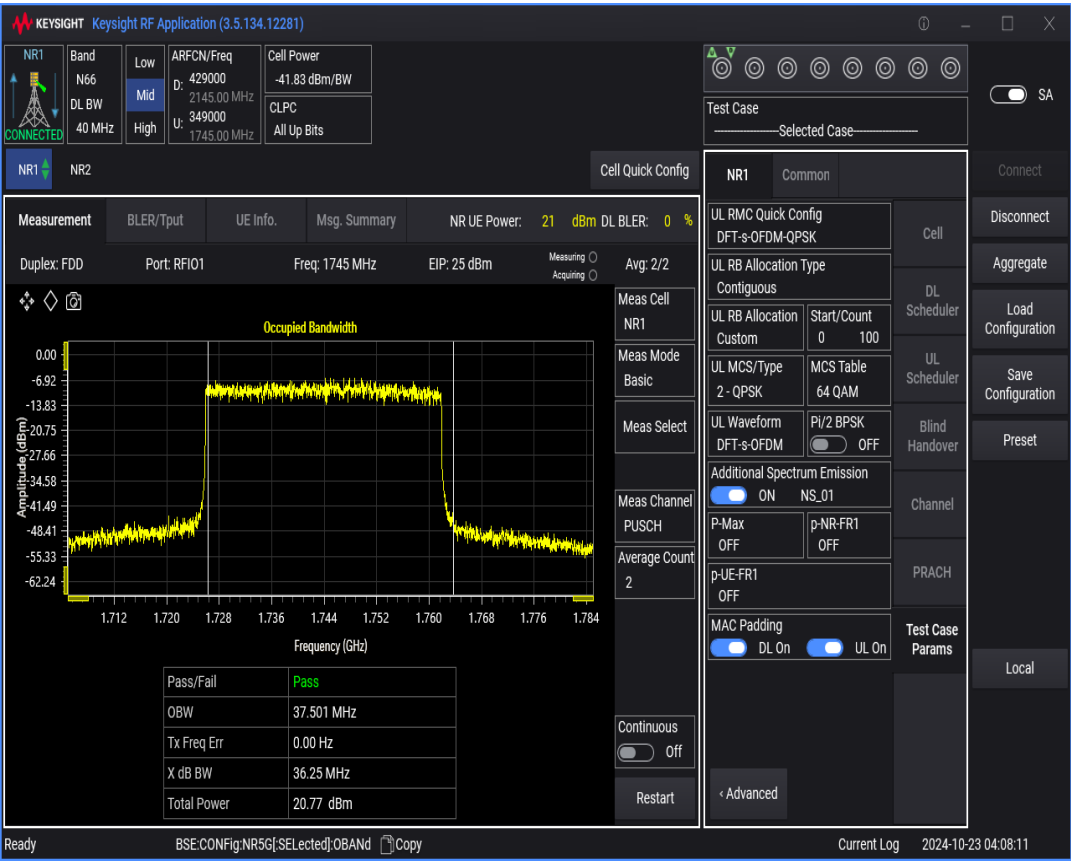
n66 SCS=30kHz DFT_QAM16 BW=40MHz Channel=349000 RB=100@0
