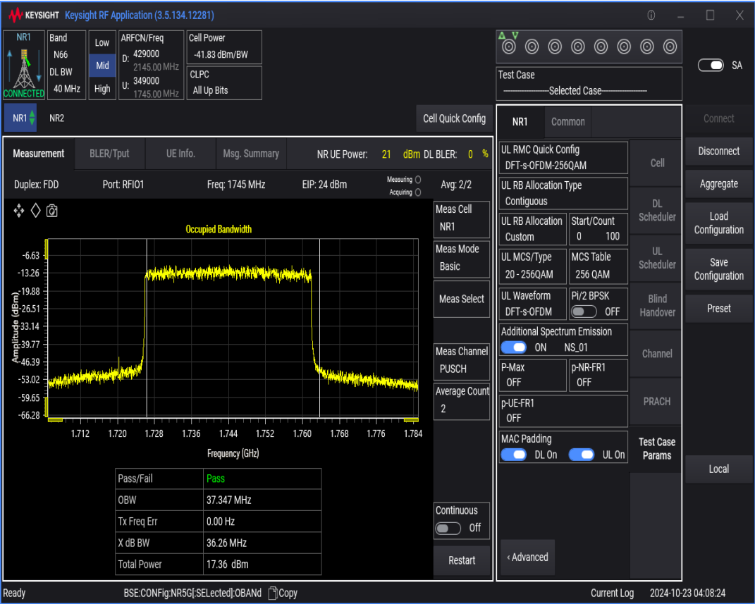
n66 SCS=30kHz DFT_QAM256 BW=40MHz Channel=349000 RB=100@0
