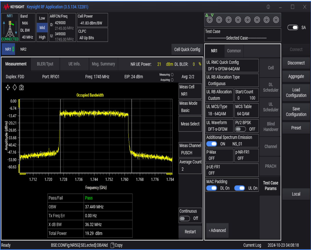
n66 SCS=30kHz DFT_QAM256 BW=40MHz Channel=349000 RB=100@0
