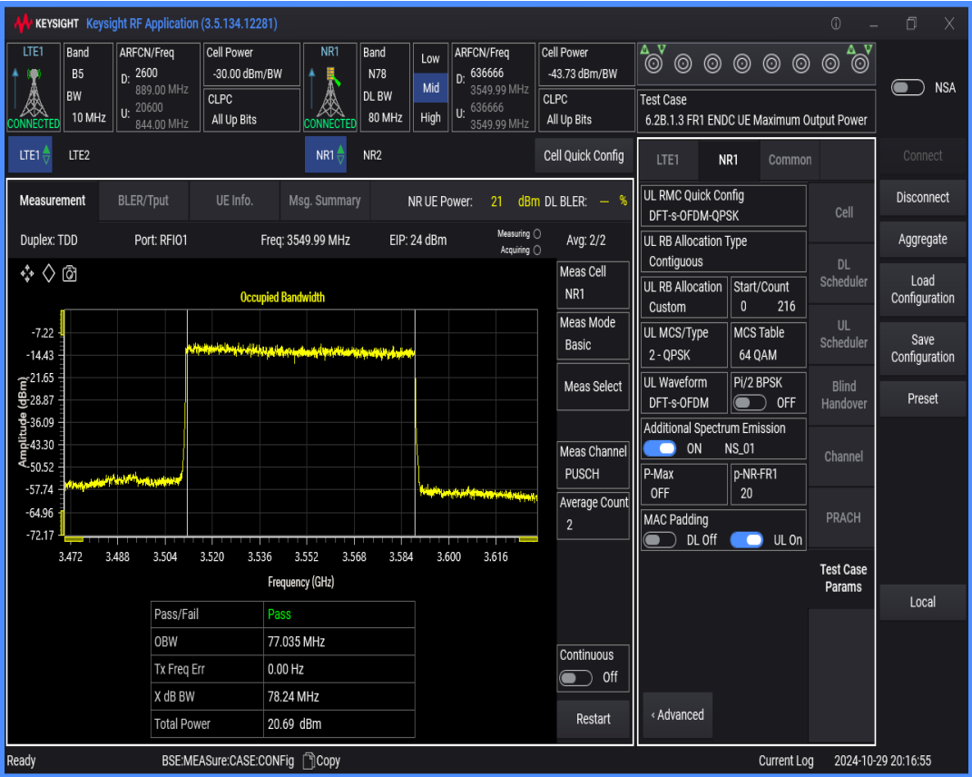
n78 SCS=30kHz DFT_QPSK BW=40MHz Channel=636666 RB=100@0
