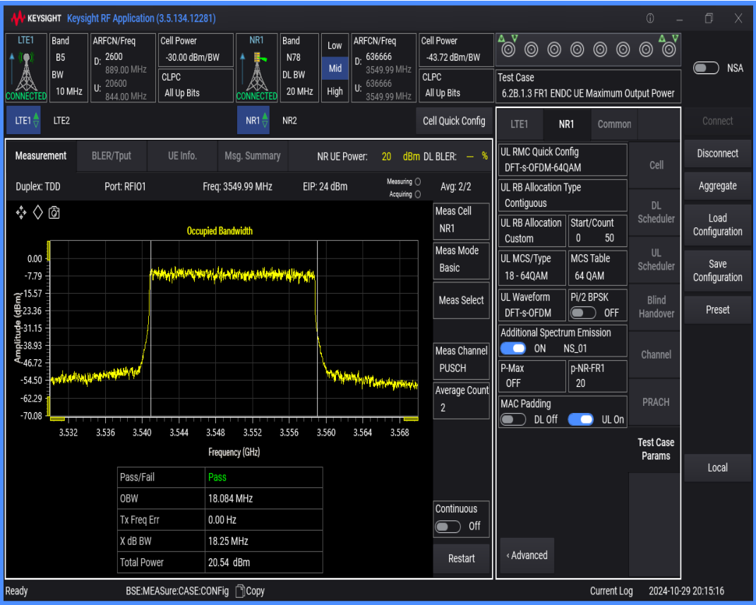
n78 SCS=30kHz DFT_QAM256 BW=90MHz Channel=636666 RB=240@0
