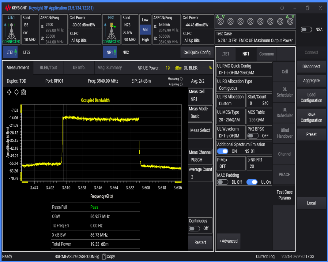
n78 SCS=30kHz DFT_QAM256 BW=80MHz Channel=636666 RB=216@0
