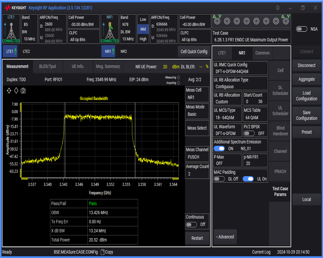
n78 SCS=30kHz DFT_QAM64 BW=10MHz Channel=636666 RB=24@0
