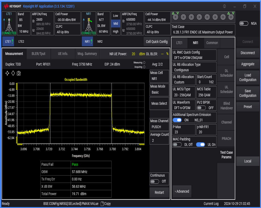
n77 SCS=30kHz DFT_QAM256 BW=80MHz Channel=650000 RB=216@0
