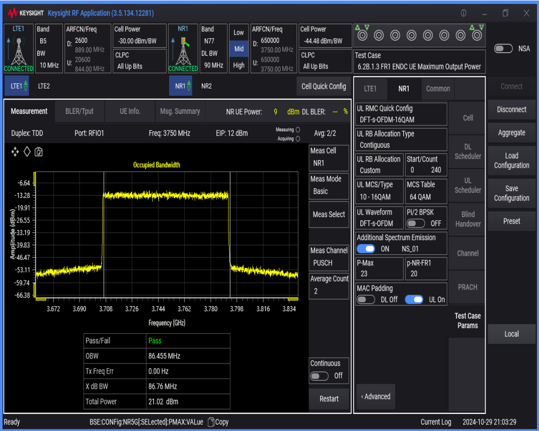
n77 SCS=30kHz DFT_QAM256 BW=15MHz Channel=650000 RB=36@0
