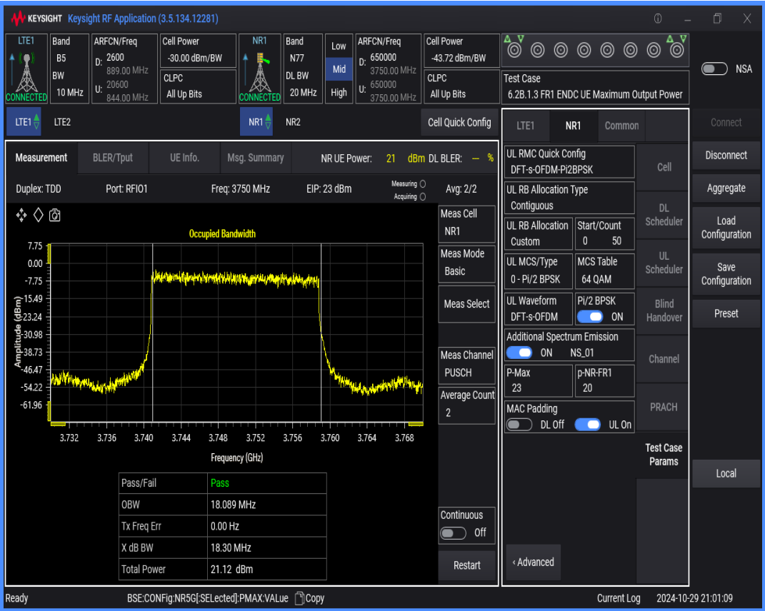
n77 SCS=30kHz DFT_BPSK BW=15MHz Channel=650000 RB=36@0
