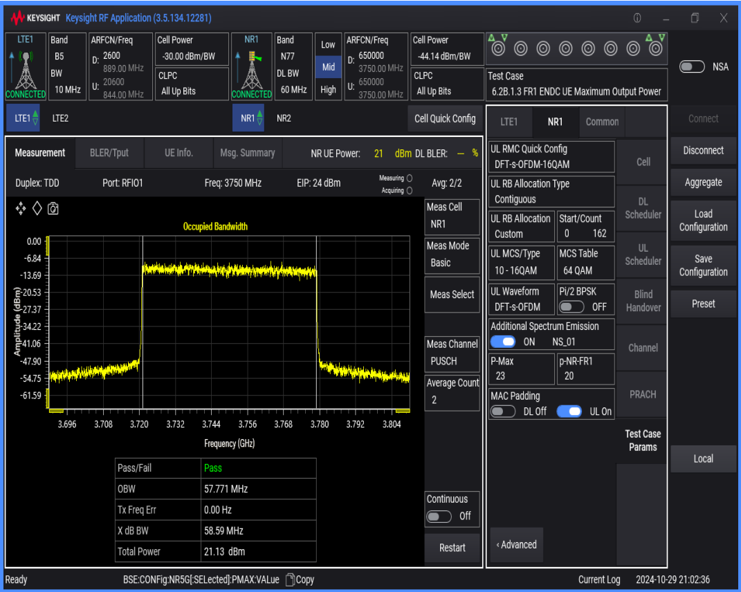
n77 SCS=30kHz DFT_QAM16 BW=50MHz Channel=650000 RB=128@0
