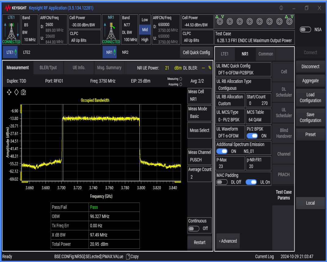
n77 SCS=30kHz DFT_BPSK BW=90MHz Channel=650000 RB=240@0
