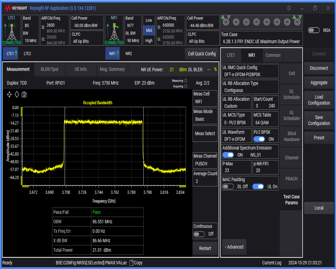
n77 SCS=30kHz DFT_BPSK BW=80MHz Channel=650000 RB=216@0
