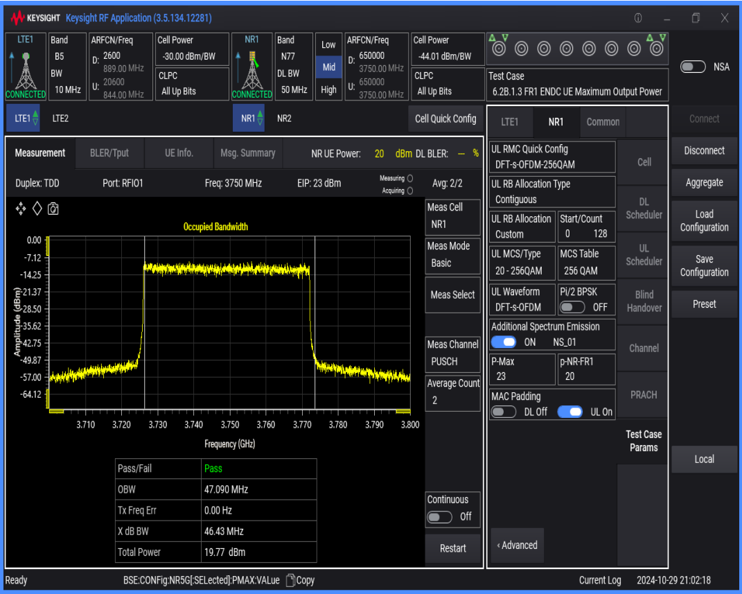
n77 SCS=30kHz DFT_QAM64 BW=50MHz Channel=650000 RB=128@0
