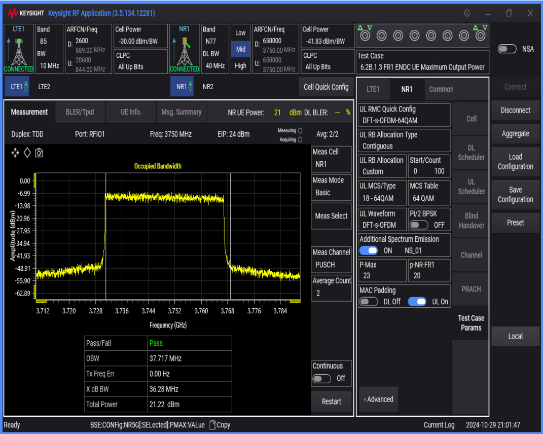
n77 SCS=30kHz DFT_QAM64 BW=20MHz Channel=650000 RB=50@0
