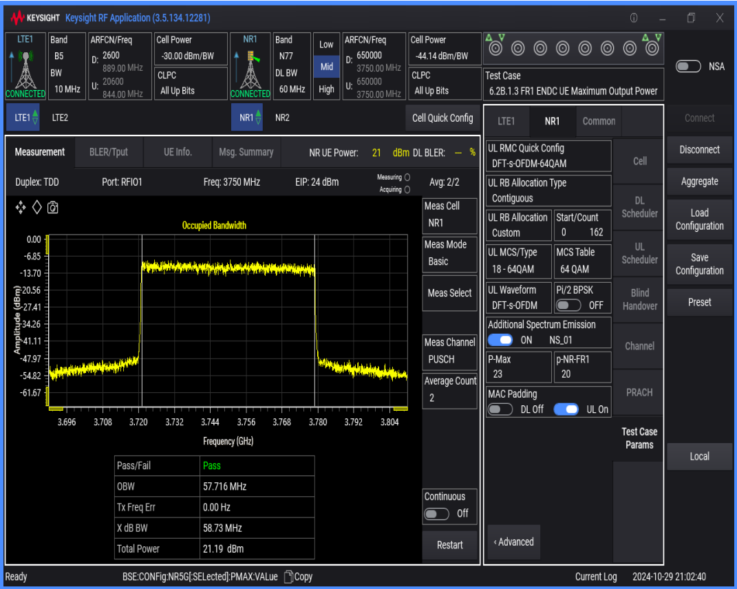
n77 SCS=30kHz DFT_QAM64 BW=50MHz Channel=650000 RB=128@0
