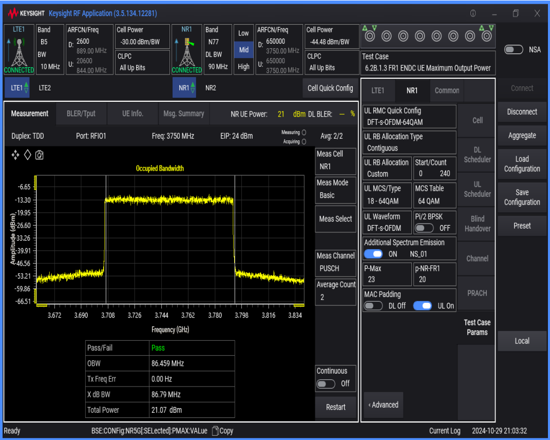
n77 SCS=30kHz DFT_QPSK BW=15MHz Channel=650000 RB=36@0
