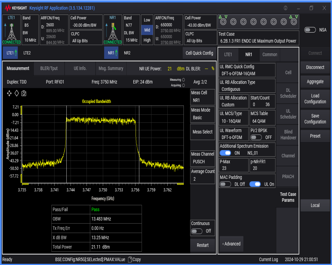
n77 SCS=30kHz DFT_QAM256 BW=10MHz Channel=650000 RB=24@0
