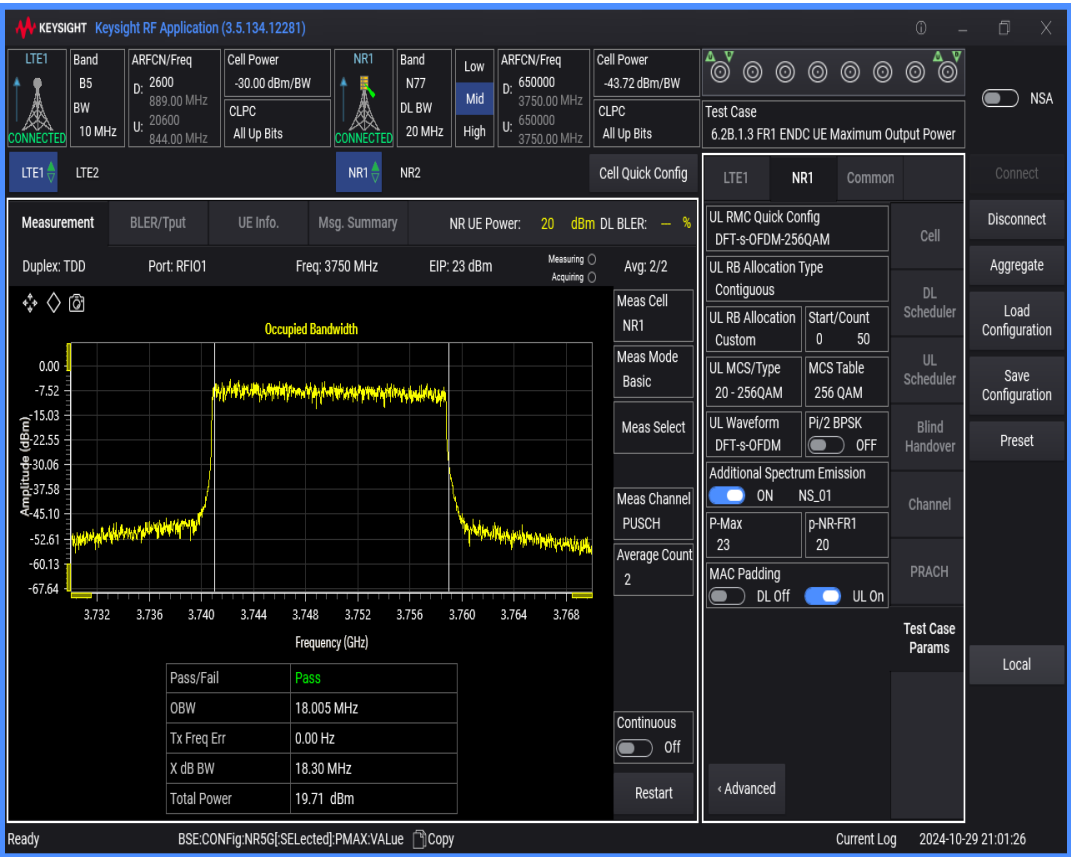
n77 SCS=30kHz DFT_QAM256 BW=15MHz Channel=650000 RB=36@0
