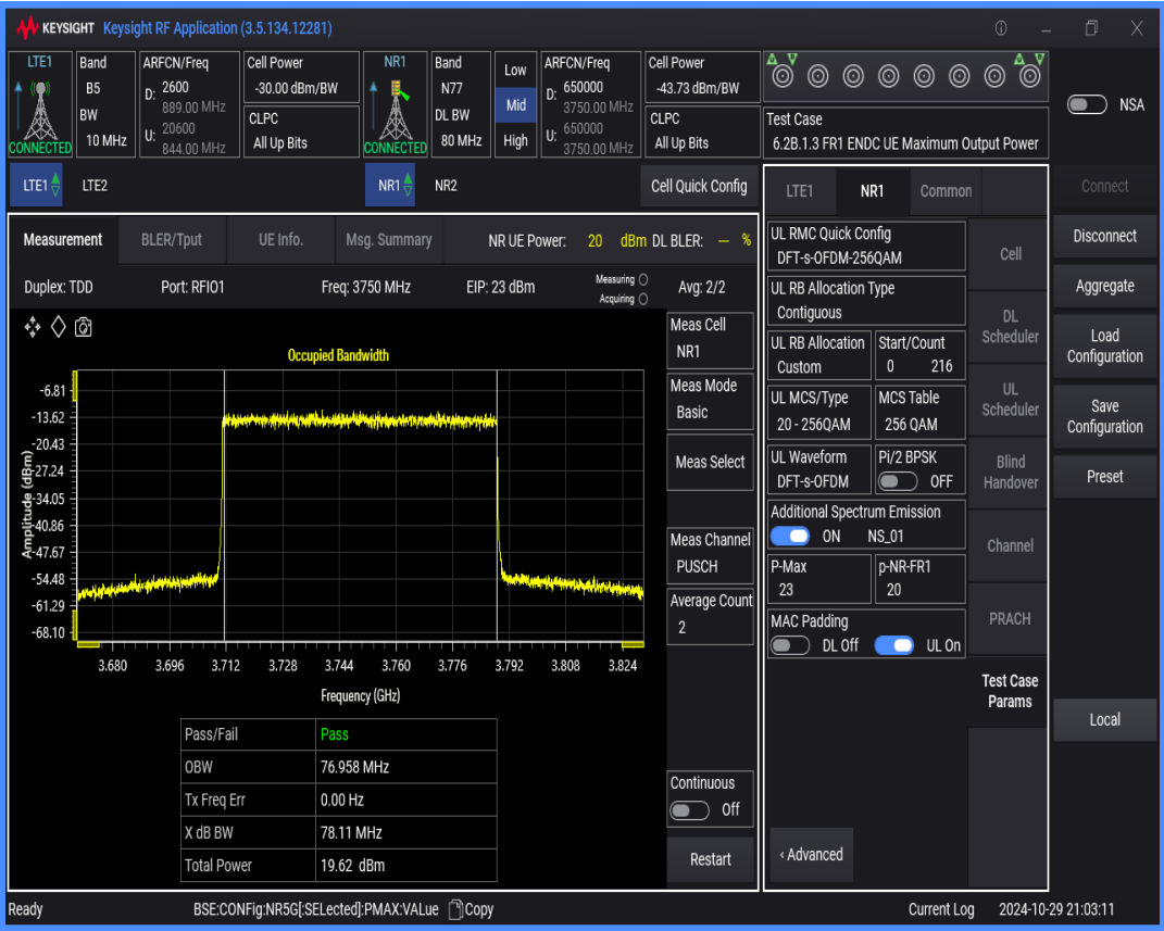
n77 SCS=30kHz DFT_QAM256 BW=60MHz Channel=650000 RB=162@0
