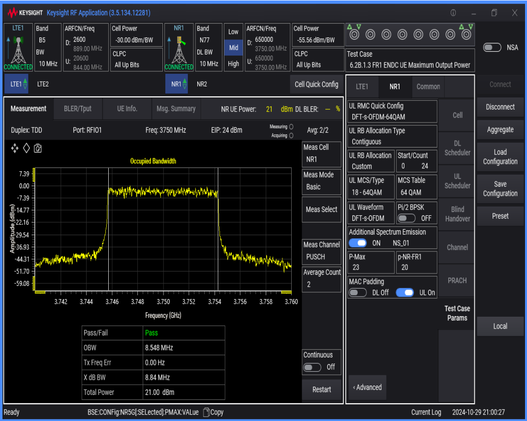
n77 SCS=30kHz DFT_QAM256 BW=50MHz Channel=650000 RB=128@0
