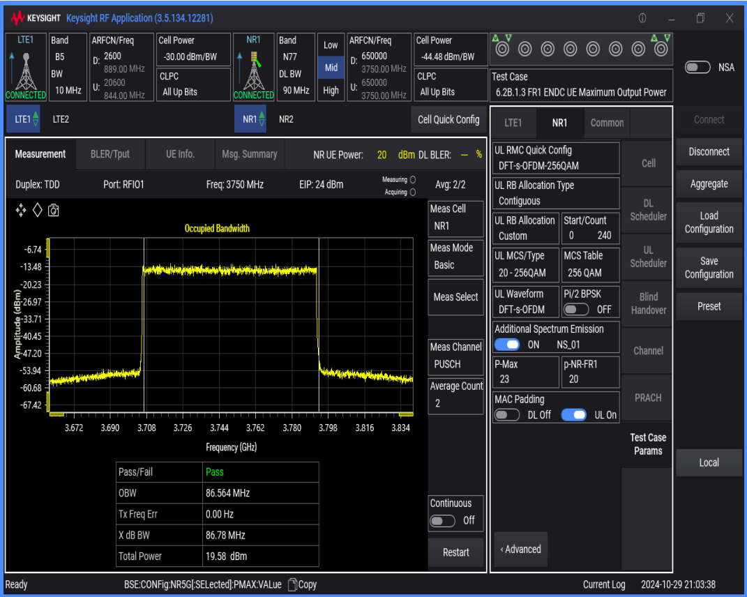
n77 SCS=30kHz DFT_QAM64 BW=15MHz Channel=650000 RB=36@0
