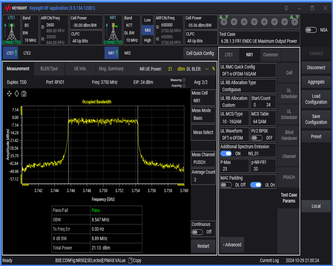
n77 SCS=30kHz DFT_BPSK BW=50MHz Channel=650000 RB=128@0
