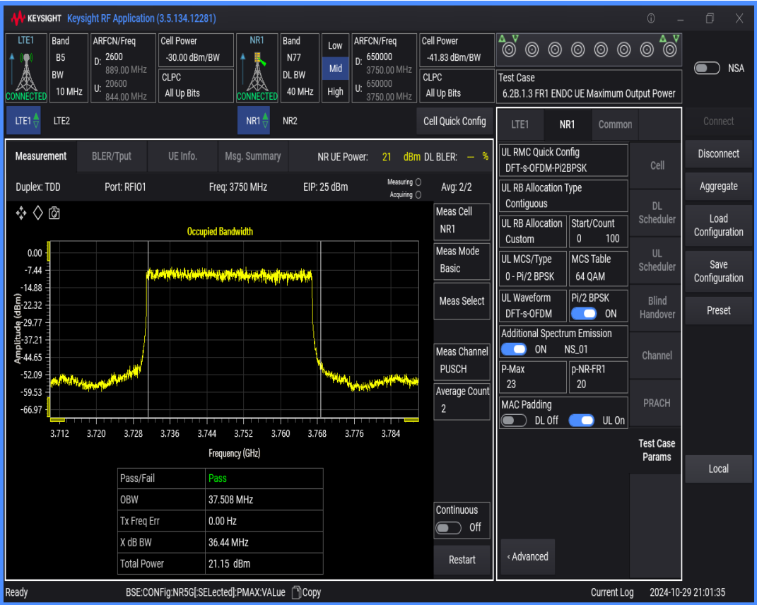
n77 SCS=30kHz DFT_BPSK BW=15MHz Channel=650000 RB=36@0
