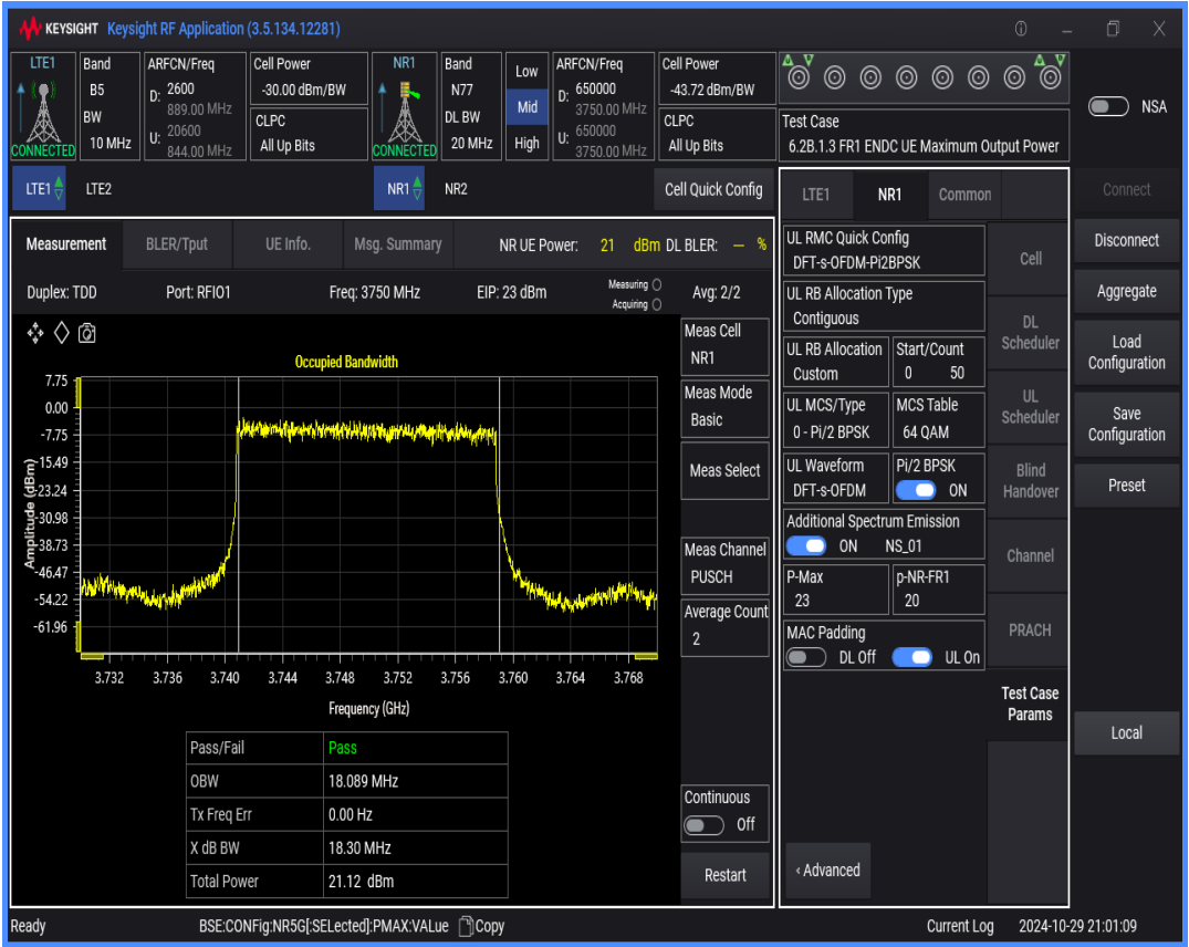
n77 SCS=30kHz DFT_BPSK BW=40MHz Channel=650000 RB=100@0
