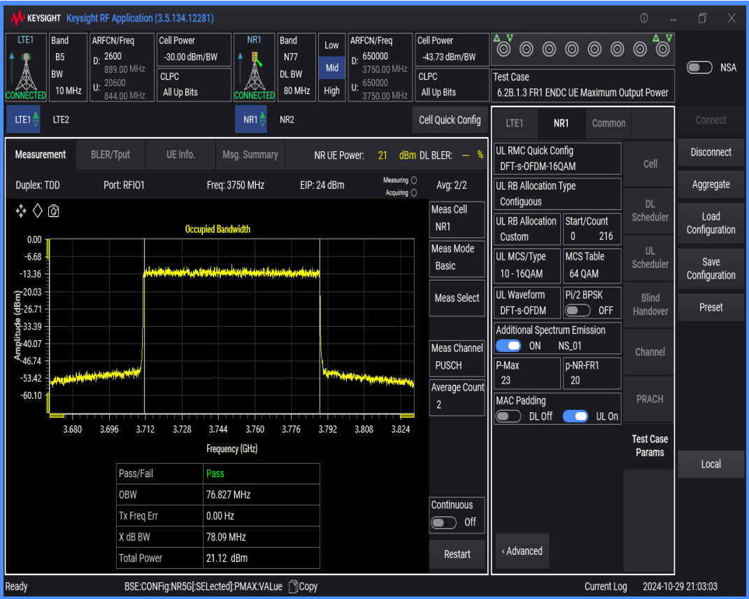
n77 SCS=30kHz DFT_QAM64 BW=100MHz Channel=650000 RB=270@0
