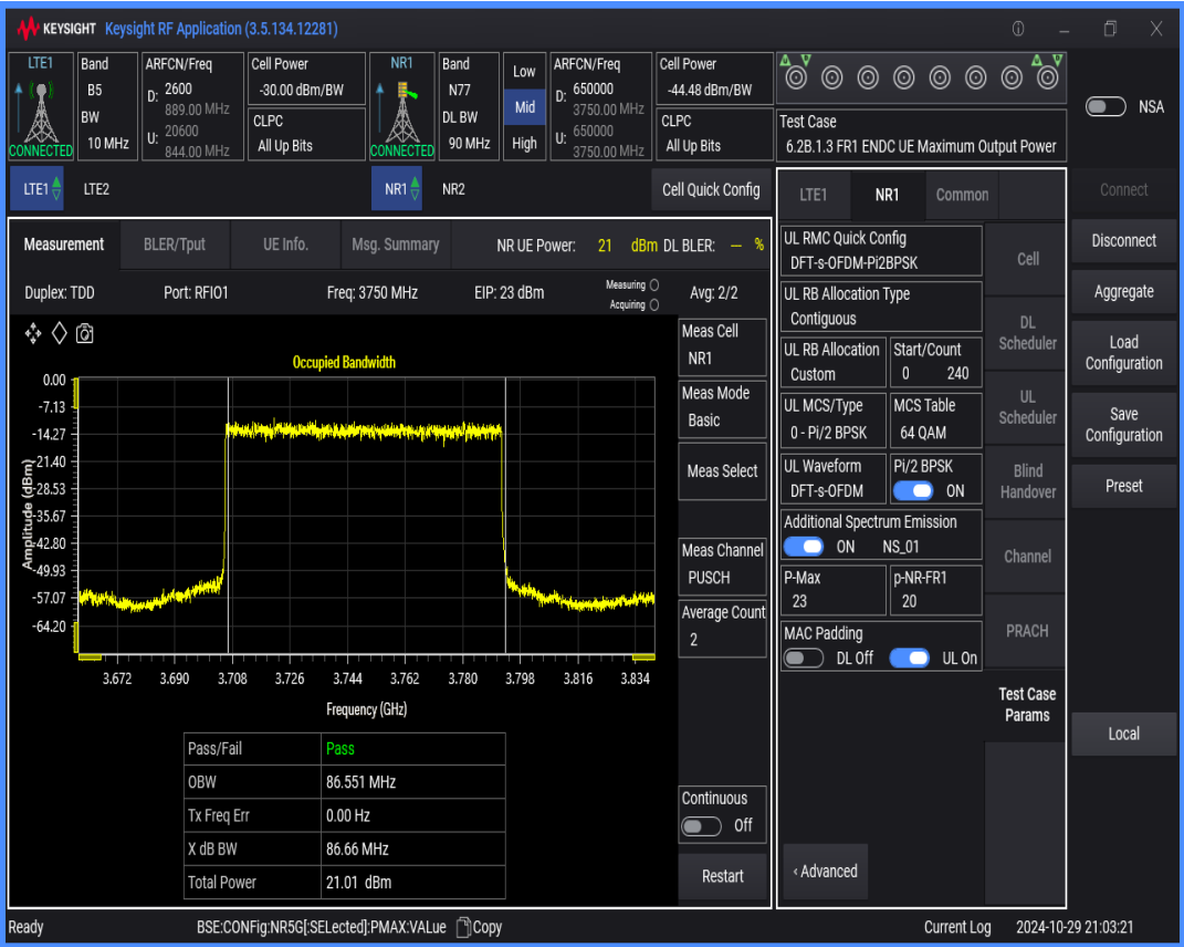
n77 SCS=30kHz DFT_QAM16 BW=100MHz Channel=650000 RB=270@0
