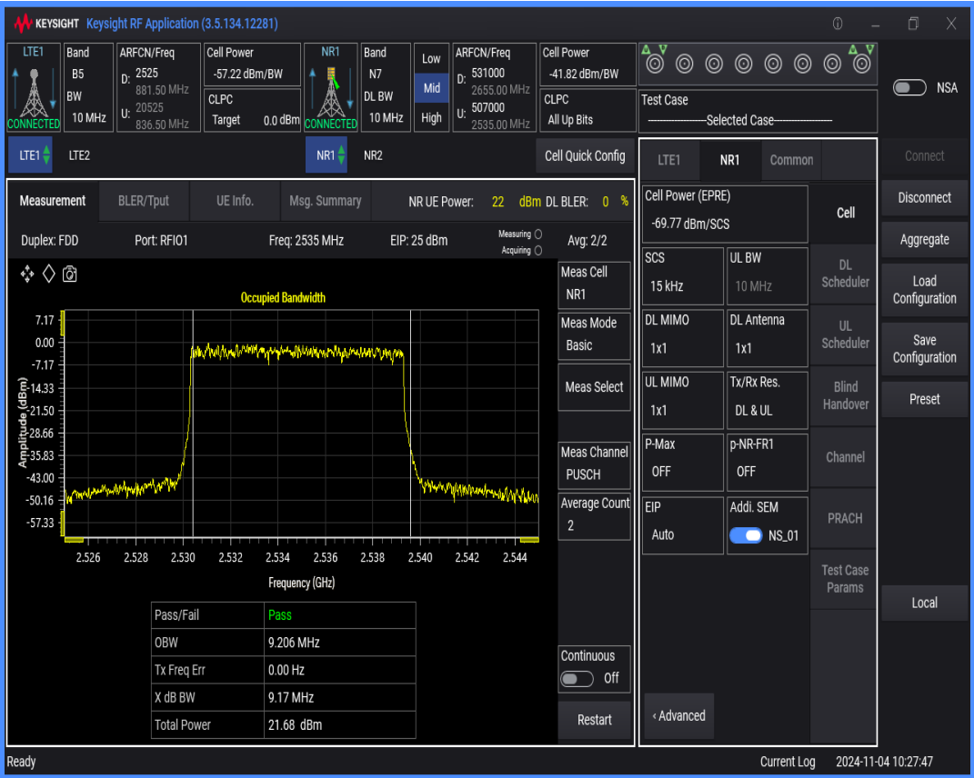
n7 SCS=15kHz DFT_QAM64 BW=5MHz Channel=507000 RB=25@0
