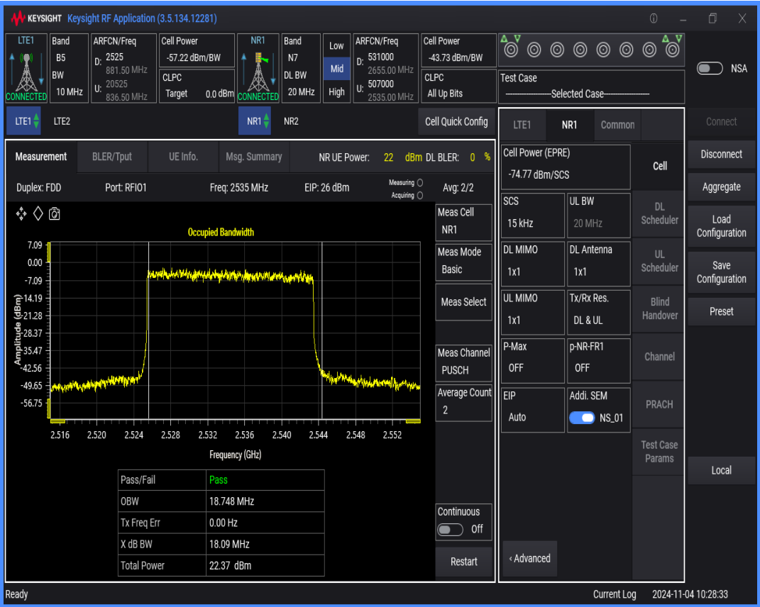
n7 SCS=15kHz DFT_BPSK BW=5MHz Channel=507000 RB=25@0
