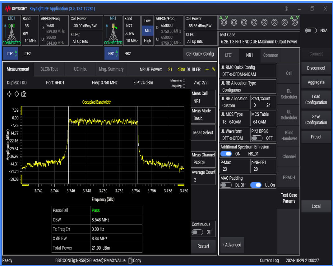
n77 SCS=30kHz DFT_QAM64 BW=100MHz Channel=650000 RB=270@0
