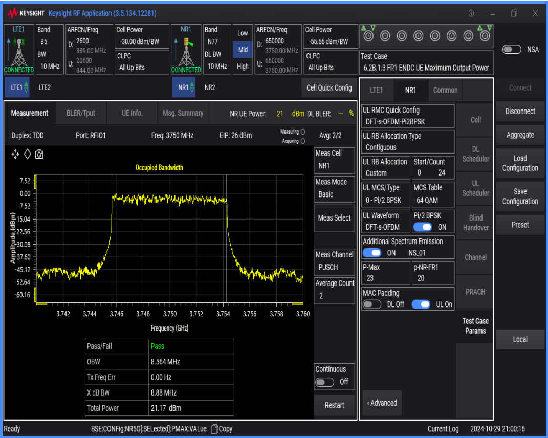
n77 SCS=30kHz DFT_BPSK BW=100MHz Channel=650000 RB=270@0
