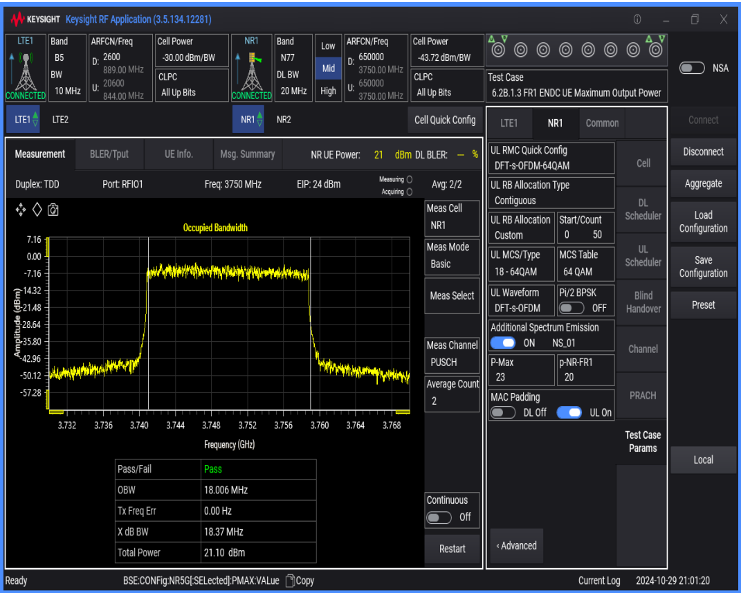
n77 SCS=30kHz DFT_QAM256 BW=50MHz Channel=650000 RB=128@0
