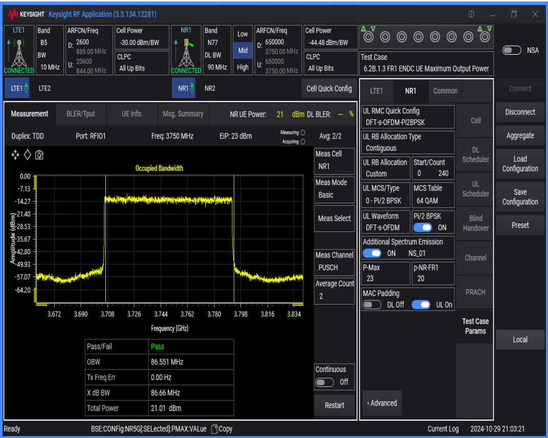
n77 SCS=30kHz DFT_QAM16 BW=10MHz Channel=650000 RB=24@0
