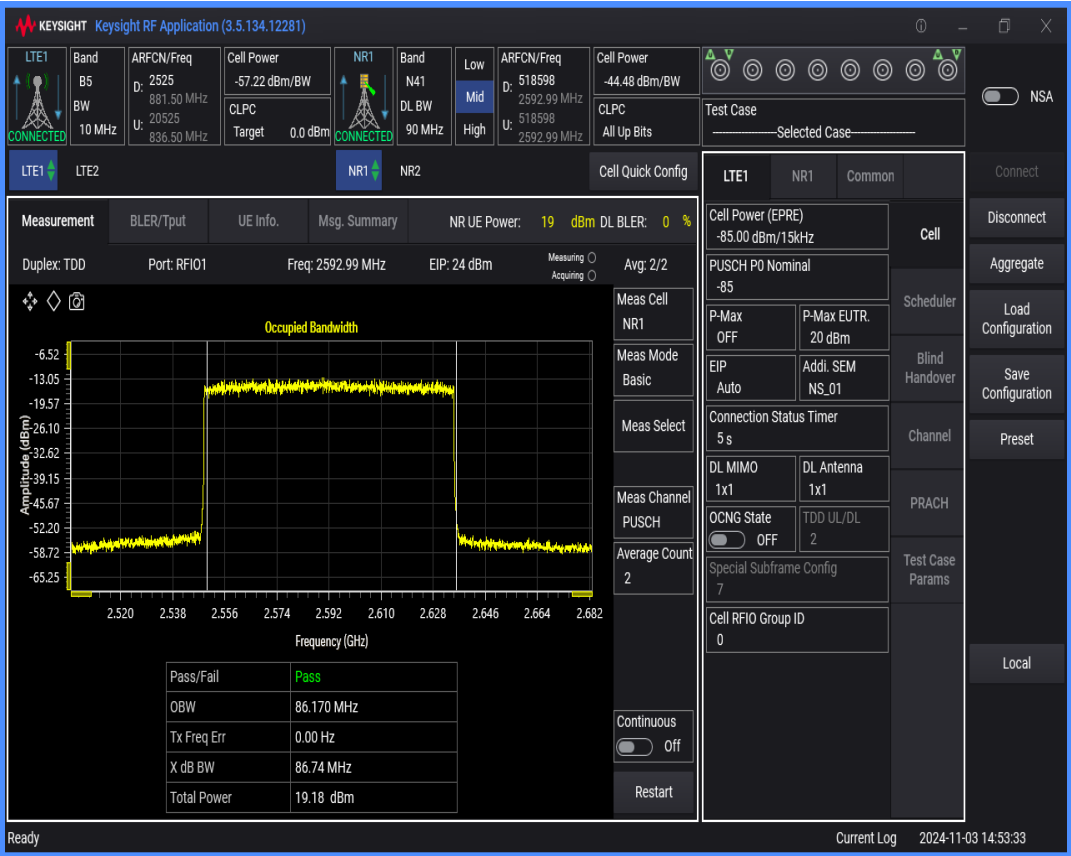
n41 SCS=30kHz DFT_QAM64 BW=100MHz Channel=518598 RB=270@0
