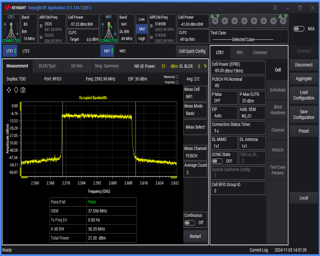
n41 SCS=30kHz DFT_QAM256 BW=90MHz Channel=518598 RB=240@0
