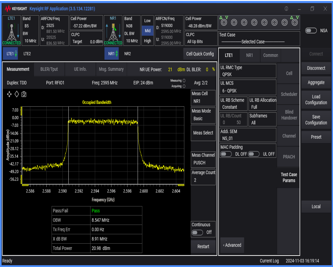
n38 SCS=30kHz DFT_QAM64 BW=15MHz Channel=519000 RB=36@0
