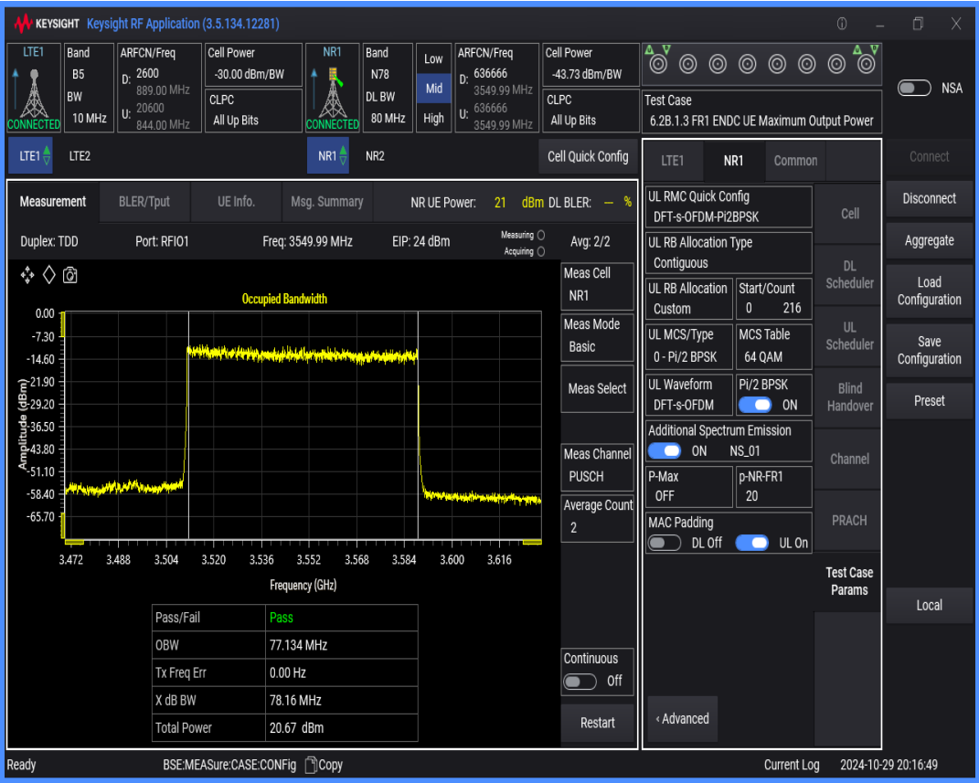
n78 SCS=30kHz DFT_QAM16 BW=100MHz Channel=636666 RB=270@0
