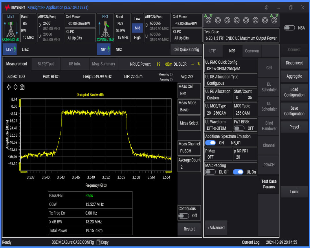
n78 SCS=30kHz DFT_QAM256 BW=50MHz Channel=636666 RB=128@0
