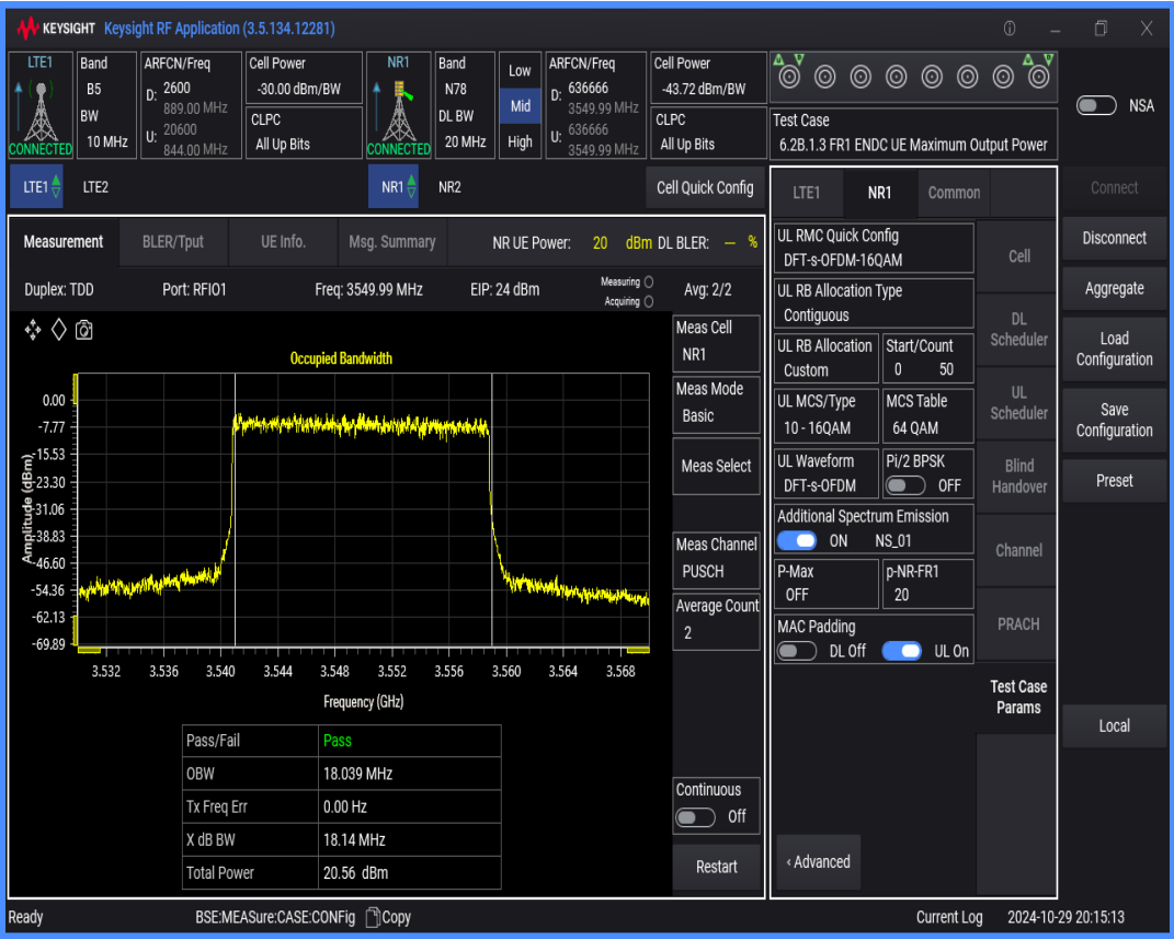
n78 SCS=30kHz DFT_QAM256 BW=10MHz Channel=636666 RB=24@0
