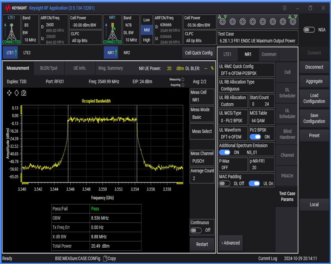
n78 SCS=30kHz DFT_BPSK BW=100MHz Channel=636666 RB=270@0
