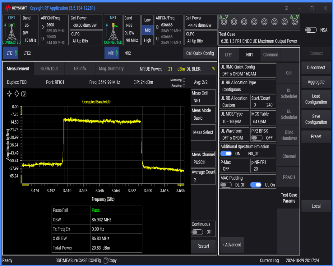
n78 SCS=30kHz DFT_QAM16 BW=50MHz Channel=636666 RB=128@0
