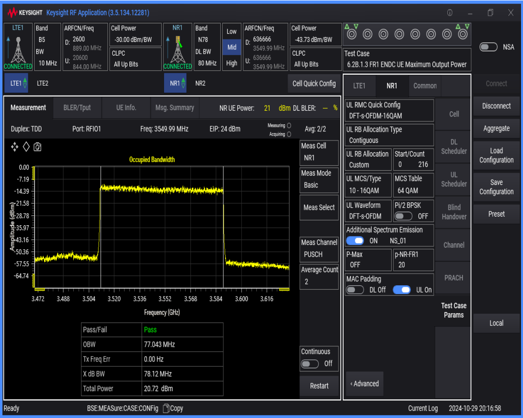
n78 SCS=30kHz DFT_QAM16 BW=60MHz Channel=636666 RB=162@0
