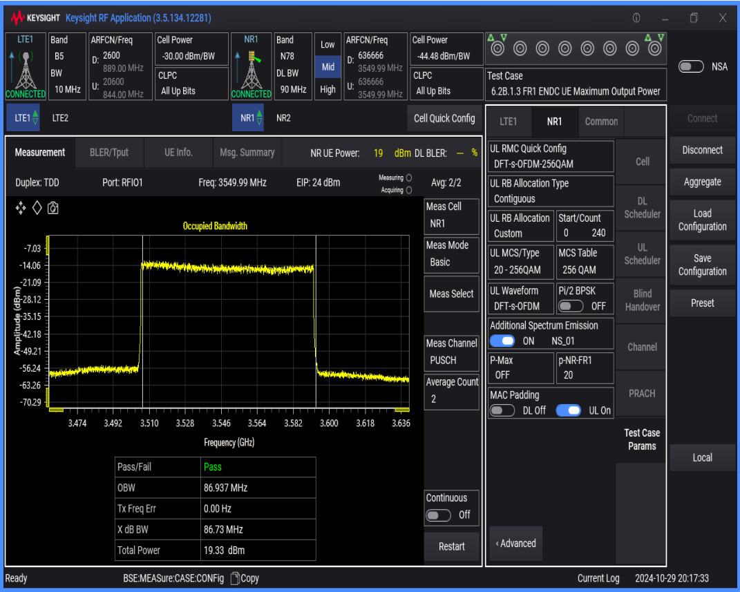
n78 SCS=30kHz DFT_QAM256 BW=80MHz Channel=636666 RB=216@0
