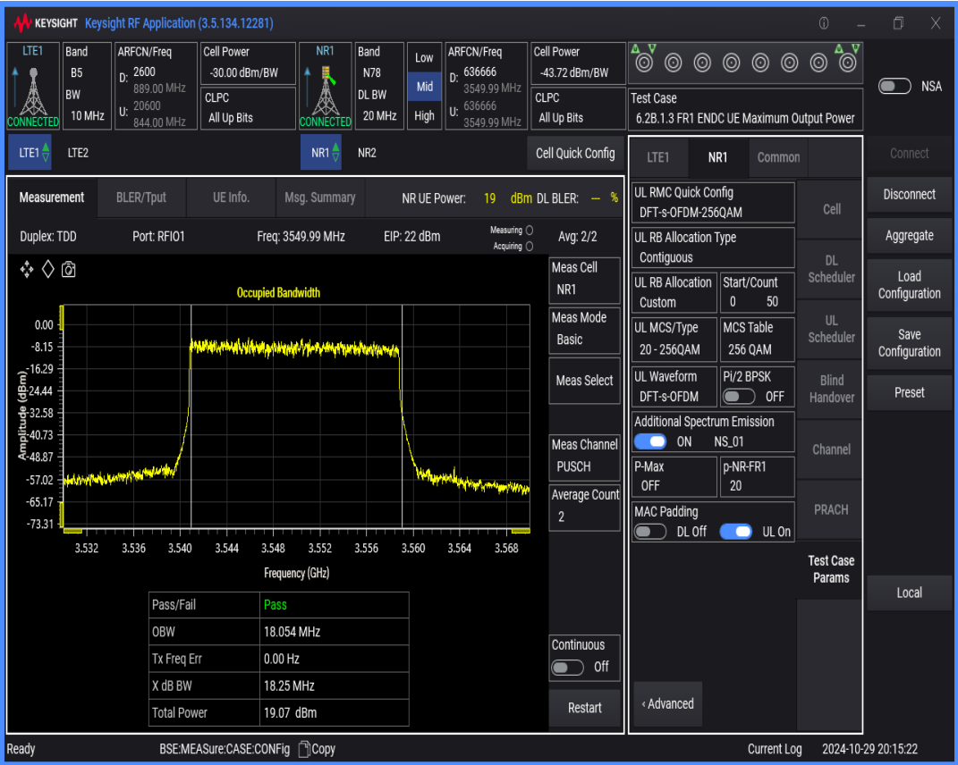
n78 SCS=30kHz DFT_QAM256 BW=15MHz Channel=636666 RB=36@0
