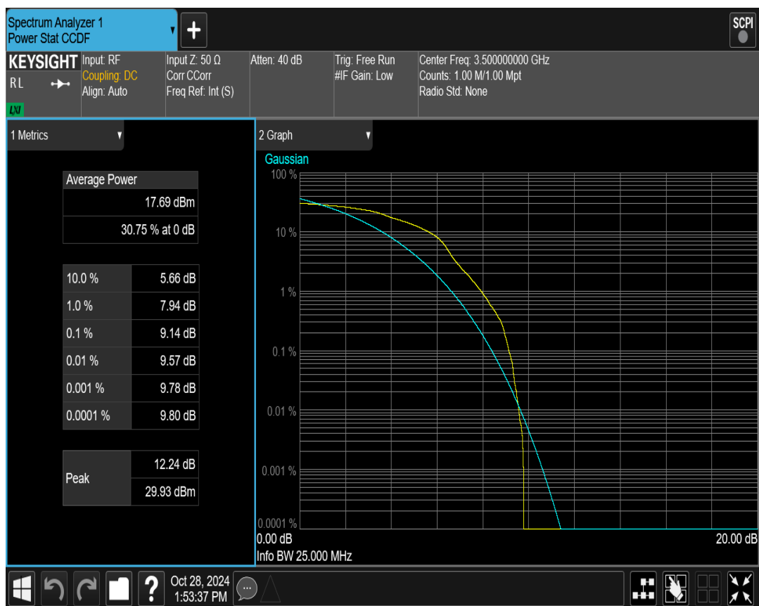
Band42(3450-3550) QAM16 BW=15MHz Channel=42590 RB Size=1 Position=#0
