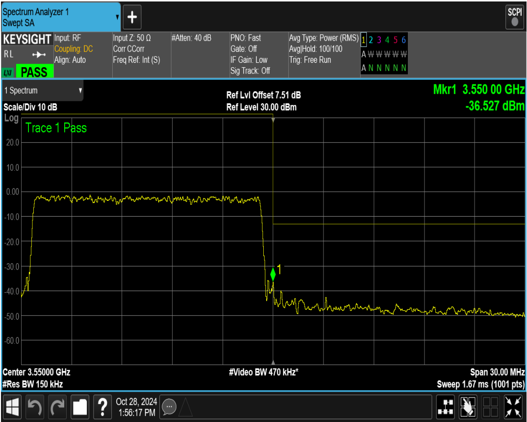
Band42(3450-3550) QPSK BW=15MHz Channel=42165 RB Size=75 Position=#0
