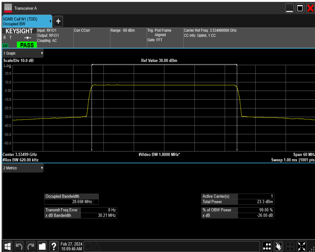
n77(3450-3550) SCS=15kHz DFT_BPSK BW=40MHz Channel=631334 RB=216@0
