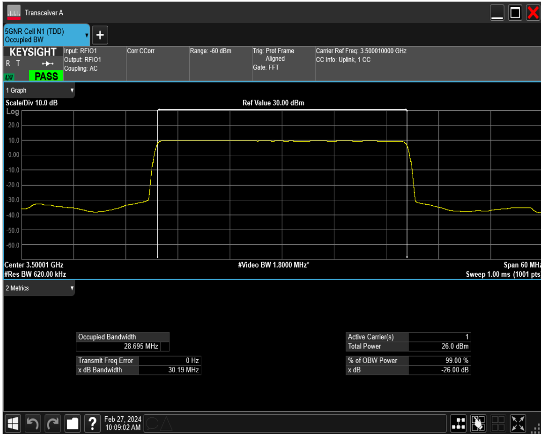
n77(3450-3550) SCS=15kHz DFT_QPSK BW=30MHz Channel=633334 RB=160@0
