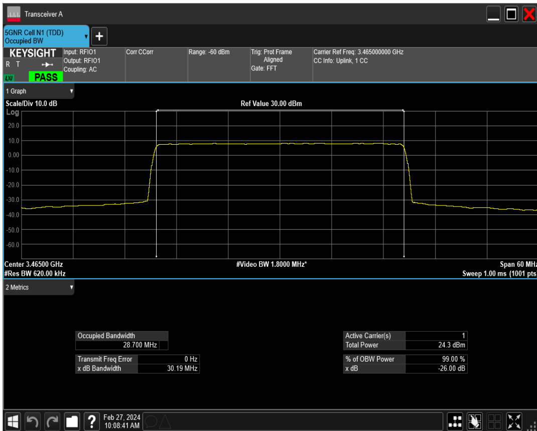
n77(3450-3550) SCS=15kHz DFT_QAM256 BW=30MHz Channel=631000 RB=160@0
