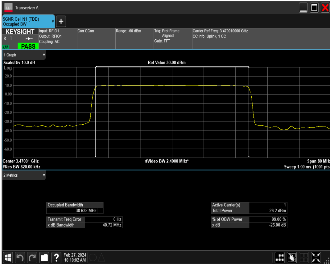
n77(3450-3550) SCS=15kHz DFT_QPSK BW=40MHz Channel=631334 RB=216@0
