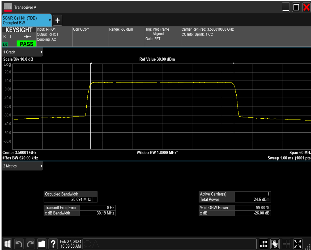
n77(3450-3550) SCS=15kHz DFT_QAM64 BW=30MHz Channel=633334 RB=160@0
