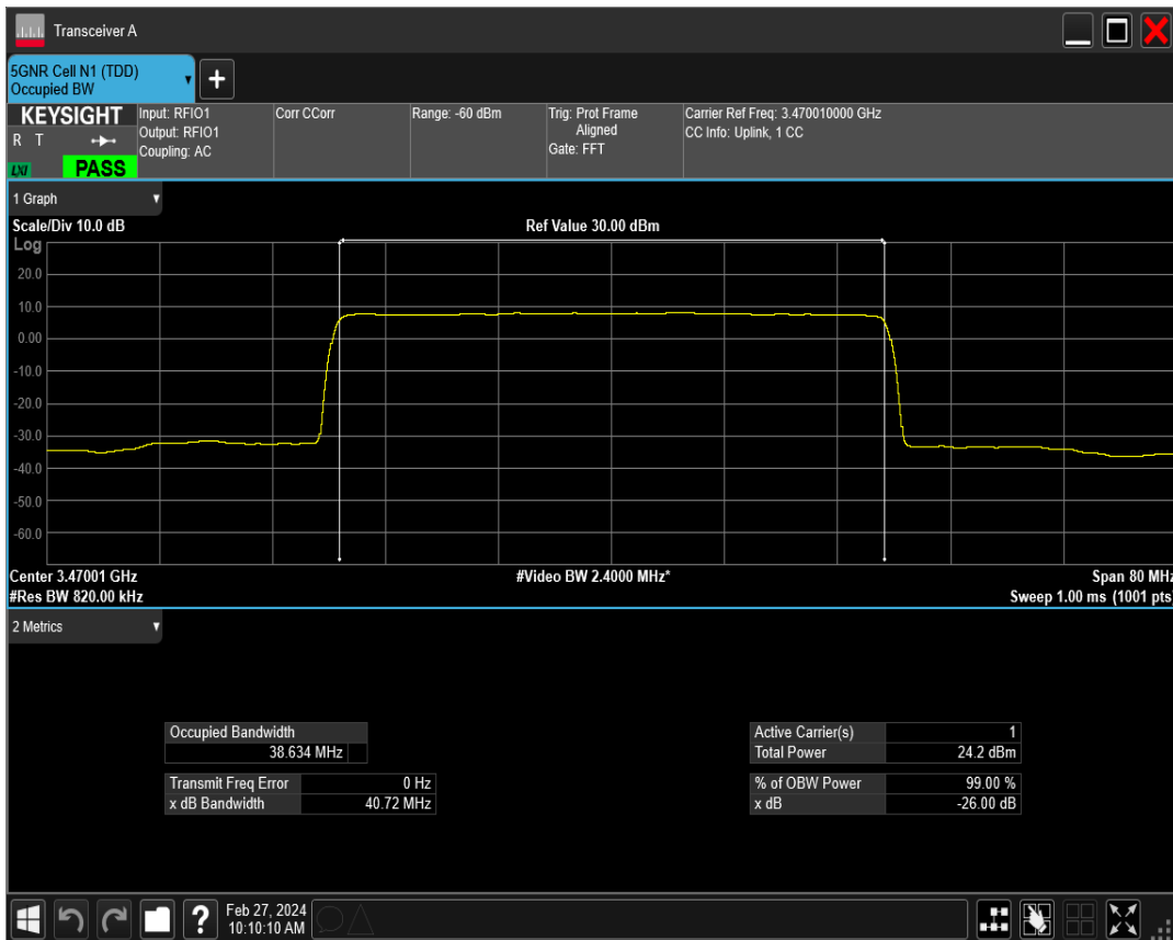
n77(3450-3550) SCS=15kHz DFT_QAM256 BW=40MHz Channel=631334 RB=216@0
