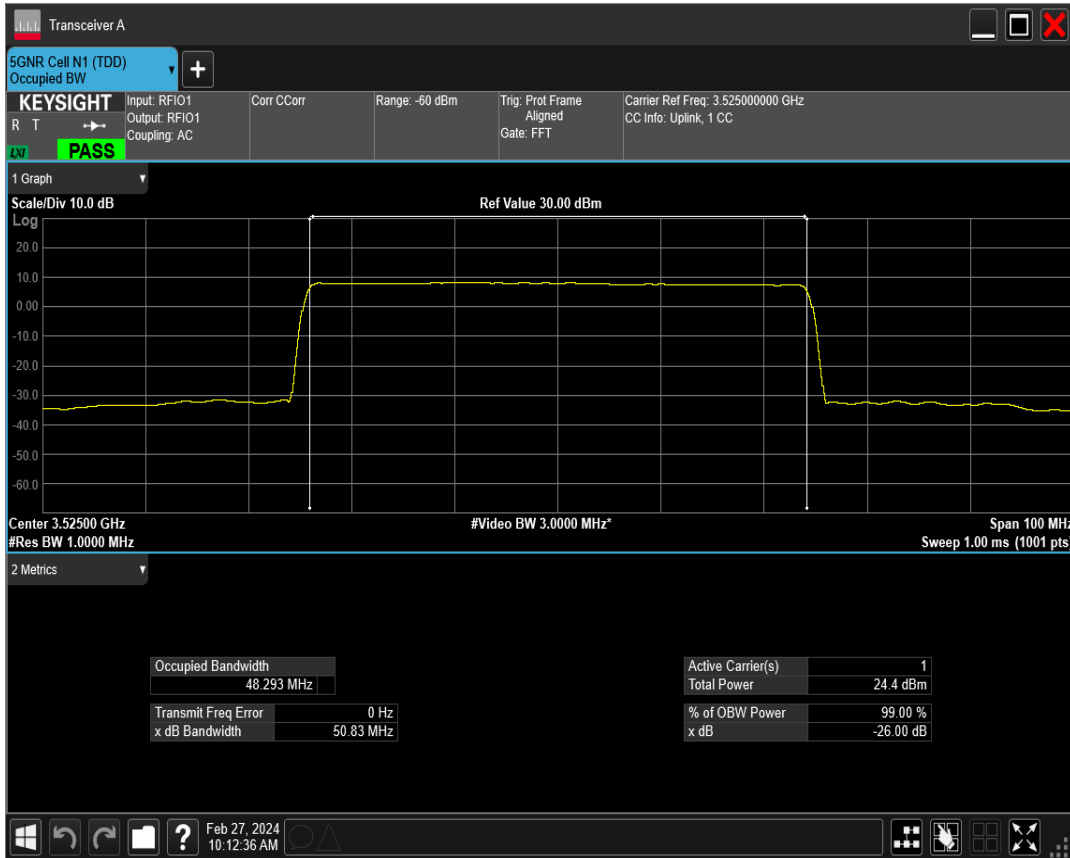
n77(3450-3550) SCS=15kHz DFT_QAM64 BW=50MHz Channel=635000 RB=270@0
