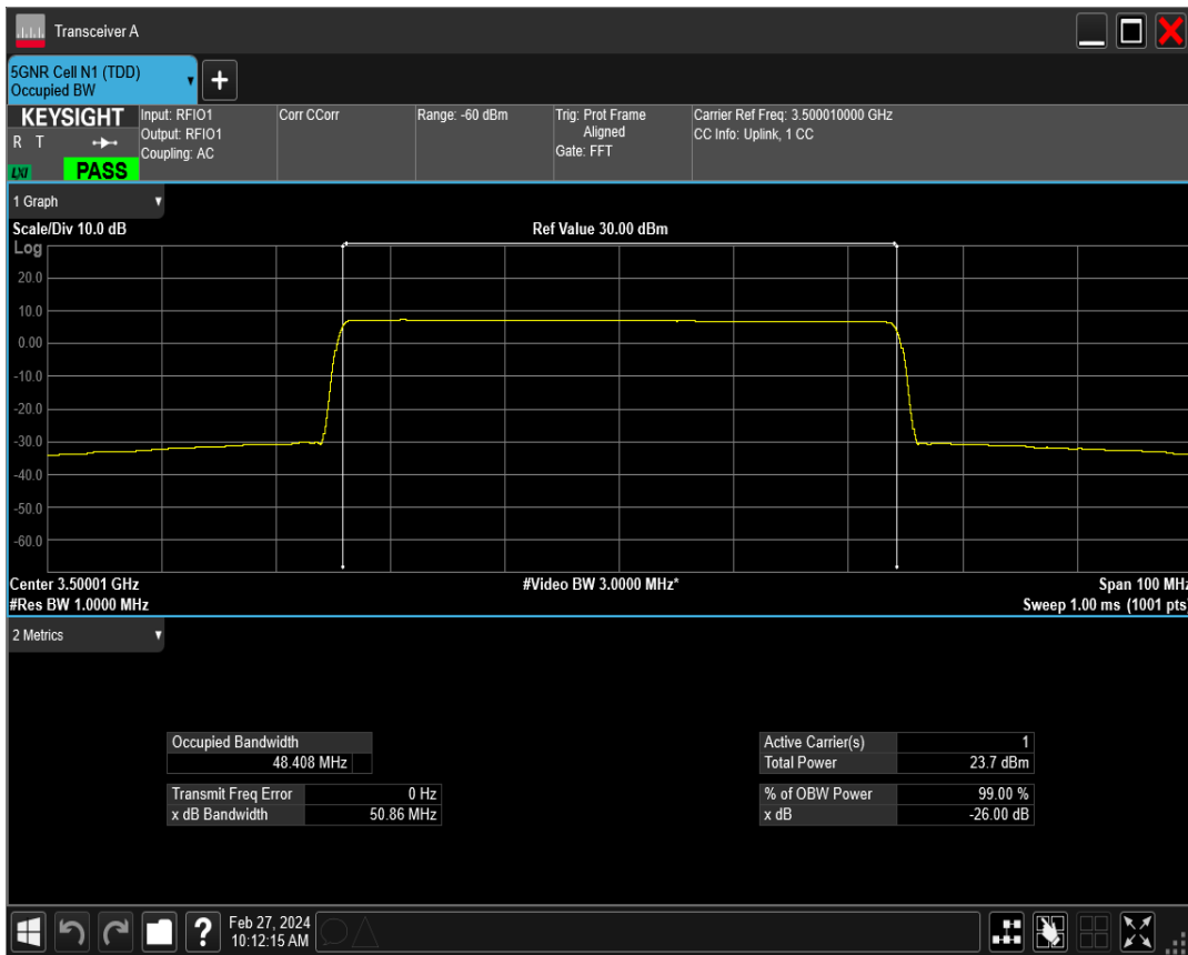
n77(3450-3550) SCS=15kHz DFT_BPSK BW=50MHz Channel=635000 RB=270@0
