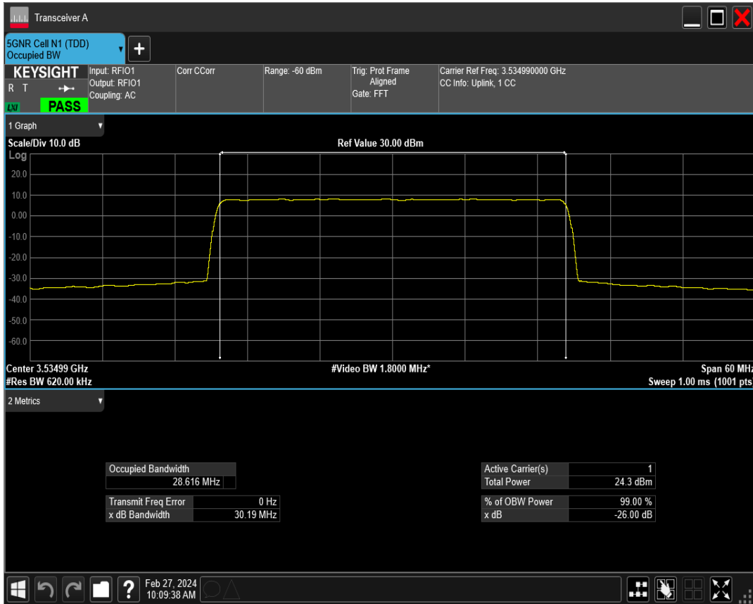
n77(3450-3550) SCS=15kHz DFT_QAM64 BW=30MHz Channel=635666 RB=160@0
