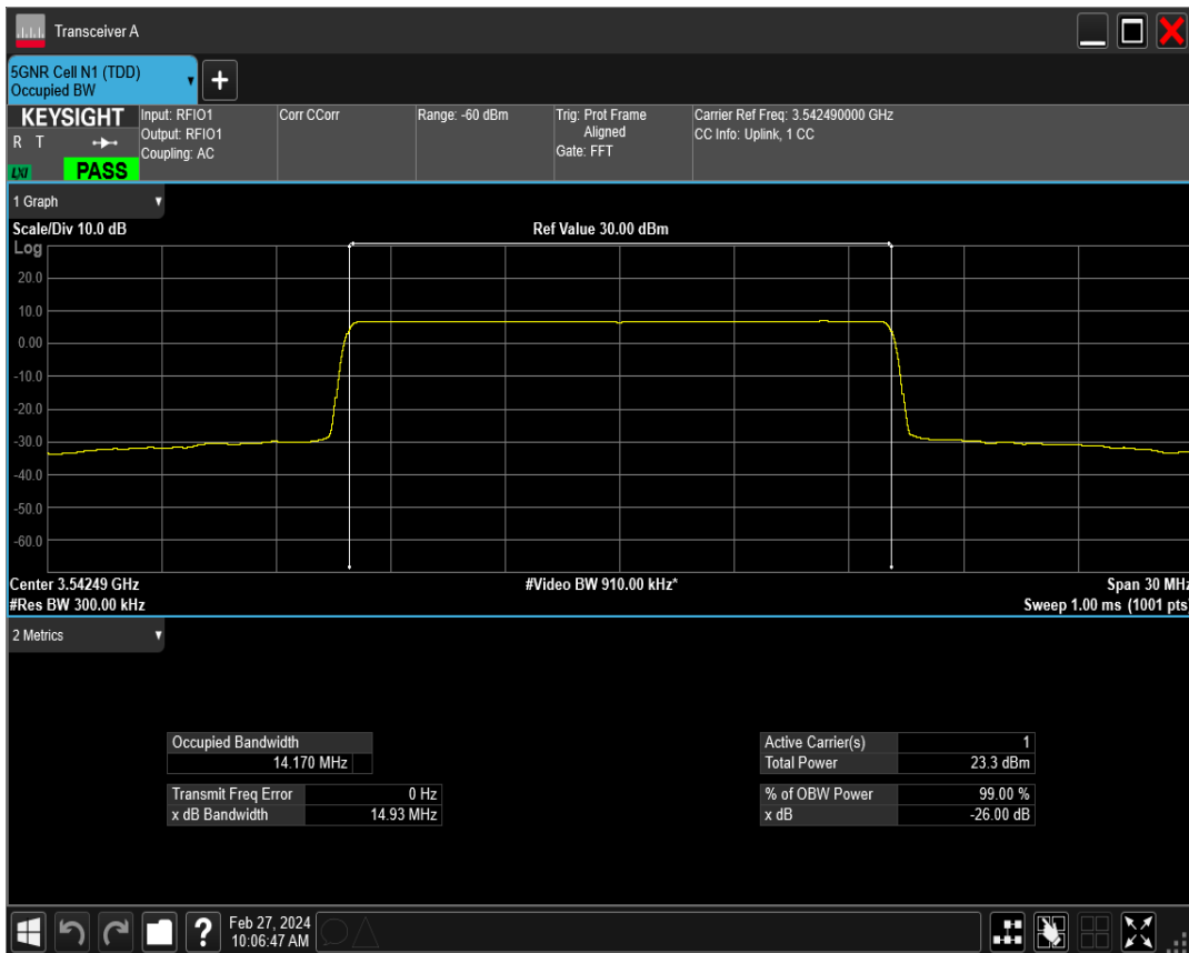
n77(3450-3550) SCS=15kHz DFT_BPSK BW=20MHz Channel=630668 RB=100@0
