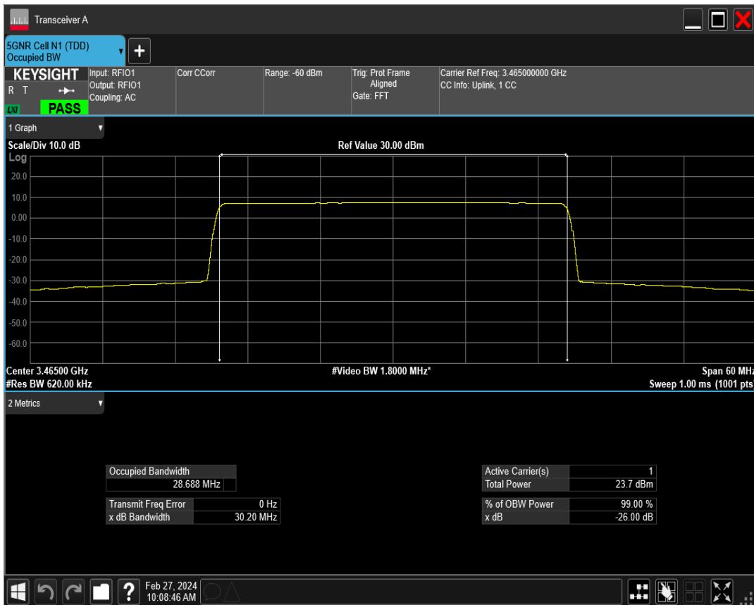
n77(3450-3550) SCS=15kHz DFT_BPSK BW=30MHz Channel=633334 RB=160@0
