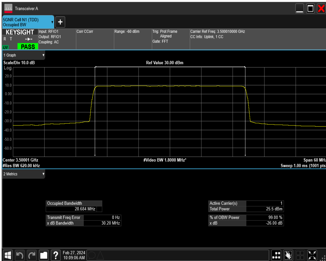
n77(3450-3550) SCS=15kHz DFT_QAM16 BW=30MHz Channel=633334 RB=160@0
