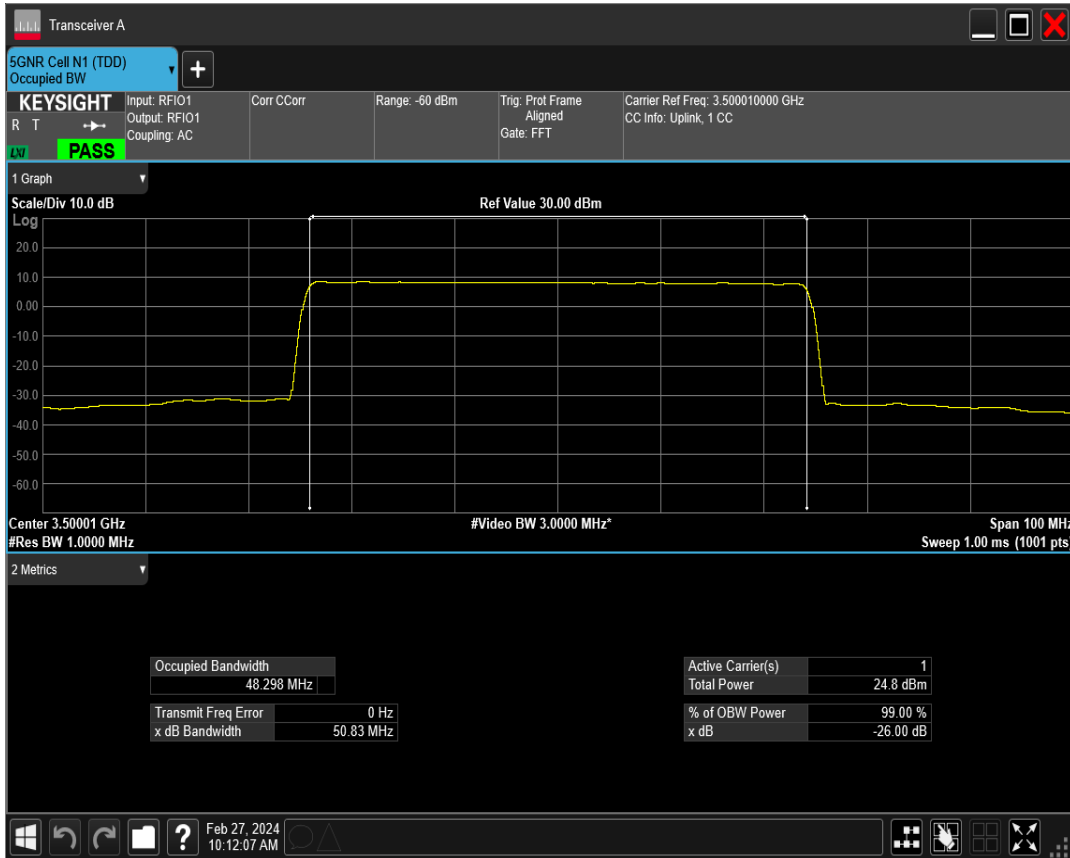
n77(3450-3550) SCS=15kHz DFT_QAM64 BW=50MHz Channel=633334 RB=270@0
