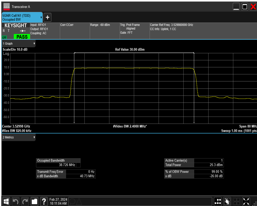
n77(3450-3550) SCS=15kHz DFT_QAM16 BW=40MHz Channel=635332 RB=216@0
