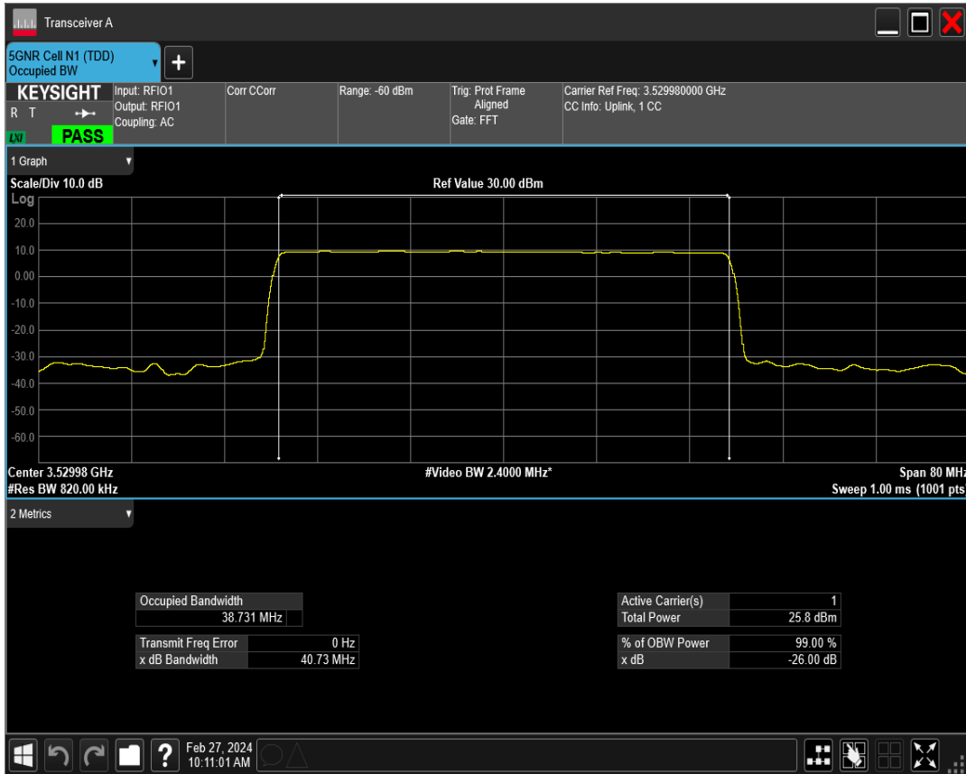
n77(3450-3550) SCS=15kHz DFT_QPSK BW=40MHz Channel=635332 RB=216@0
