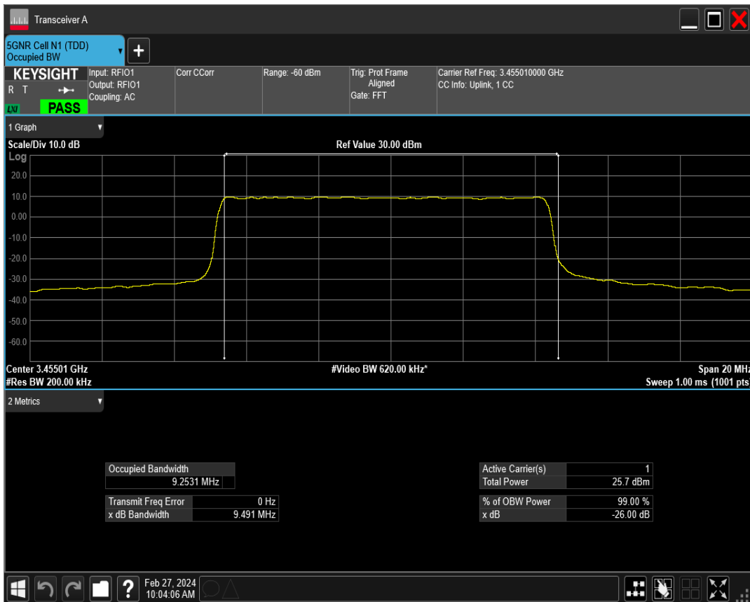
n77(3450-3550) SCS=15kHz DFT_QAM16 BW=10MHz Channel=630334 RB=50@0
