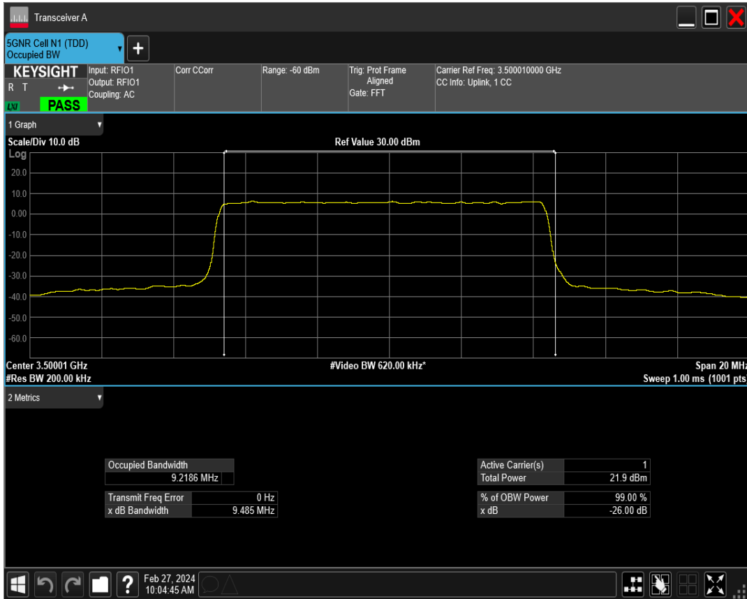
n77(3450-3550) SCS=15kHz CP_QPSK BW=10MHz Channel=633334 RB=52@0
