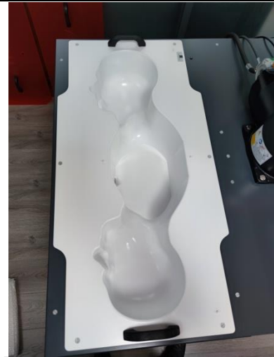
Fig. 8.7 Photo of SAM Phantom
