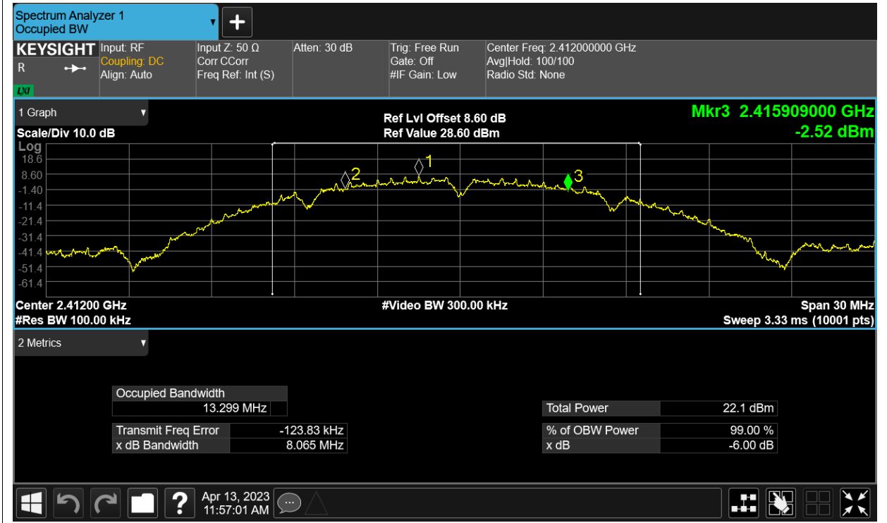
-6dB Bandwidth NVNT b 2437MHz Ant1
