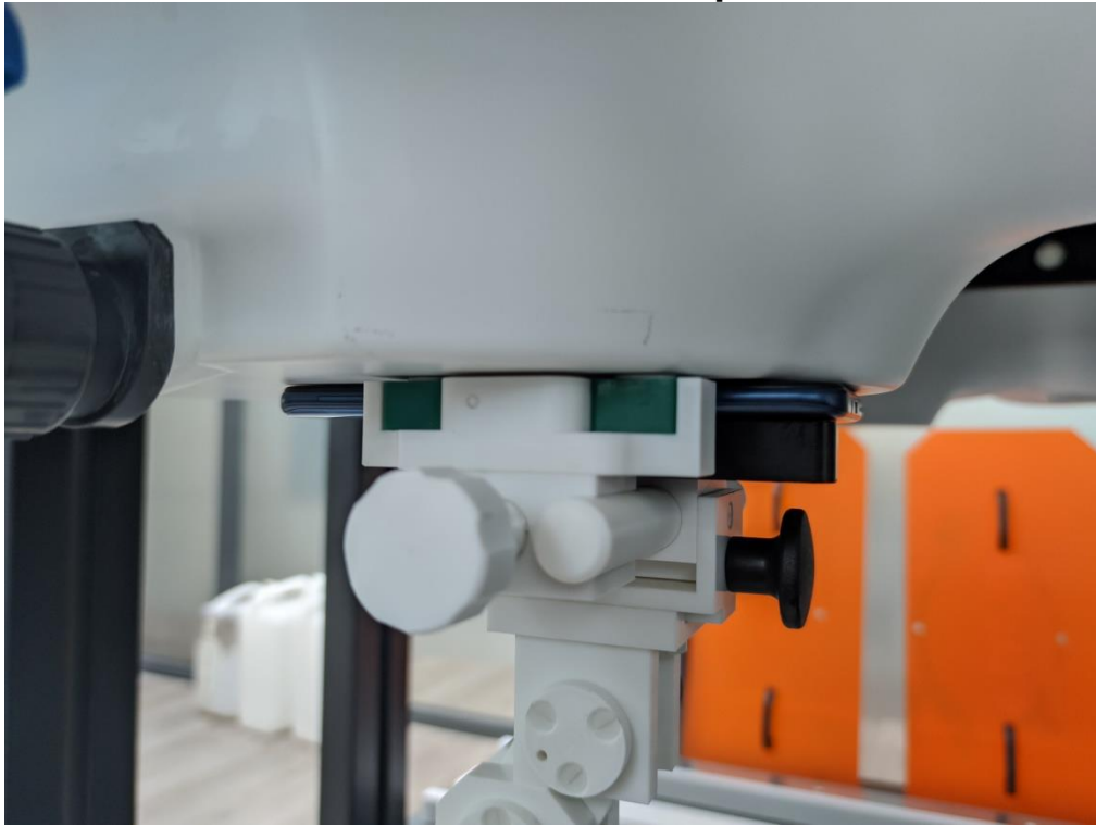
DUT with device holder (DUT direct contact with the phantom)
