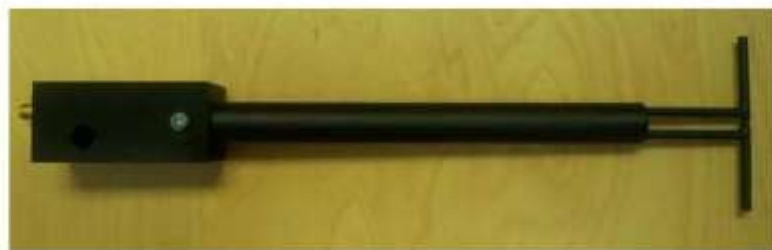
Figure 1 – MVG COMOSAR Validation Dipole
