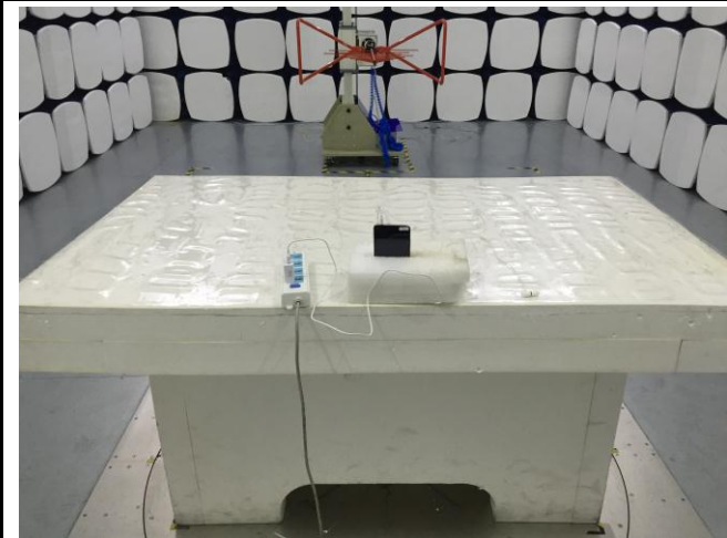
Conducted Emissions Test Setup Front View
