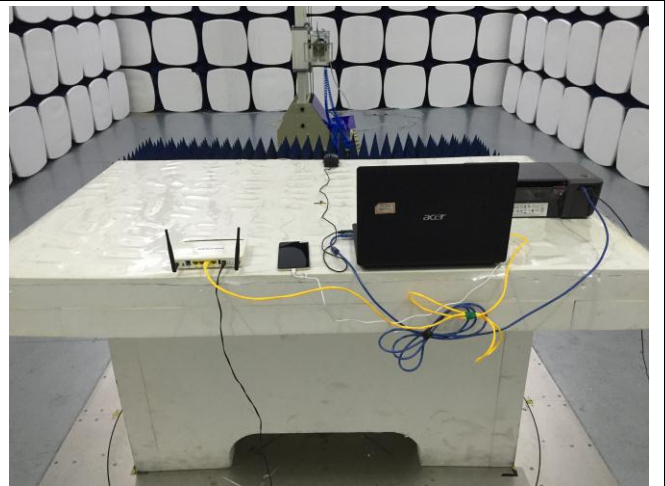
Radiated Emissions Test Setup Above 1GHz
