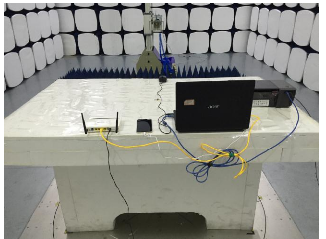
Radiated Emissions Test Setup Above 1GHz
