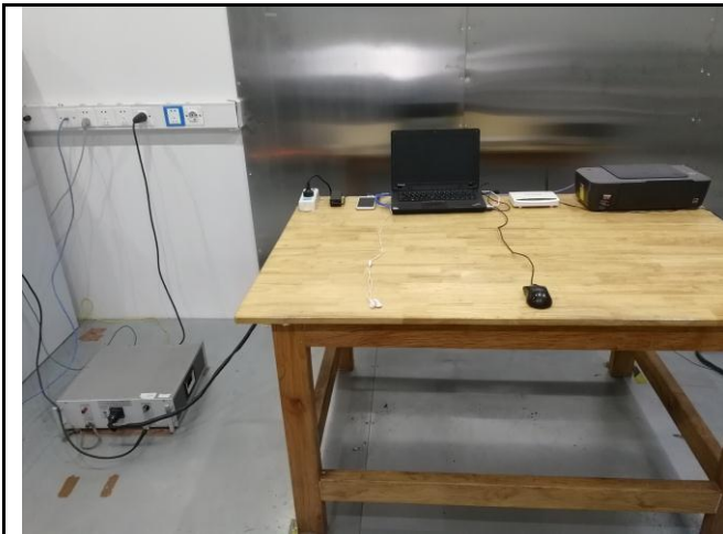
Conducted Emissions Test Setup – Front View
