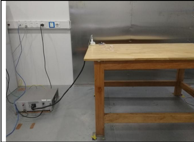
Conducted Emissions Test Setup Front View
