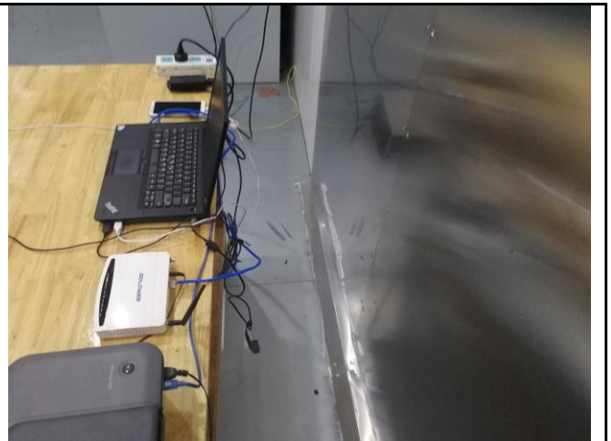
Conducted Emissions Test Setup – Side View
