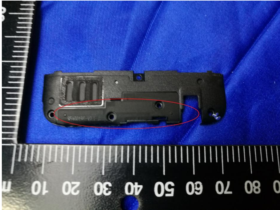
GSM/PCS/UMTS/LTE - Antenna View
