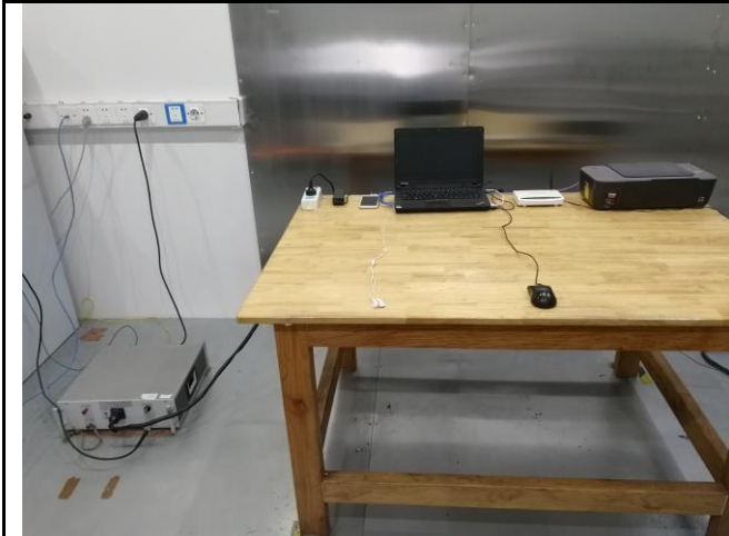
Conducted Emissions Test Setup – Front View
