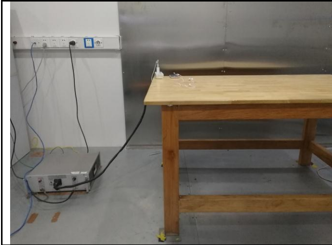
Conducted Emissions Test Setup Front View
