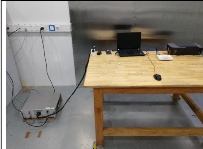
Conducted Emissions Test Setup – Front View
