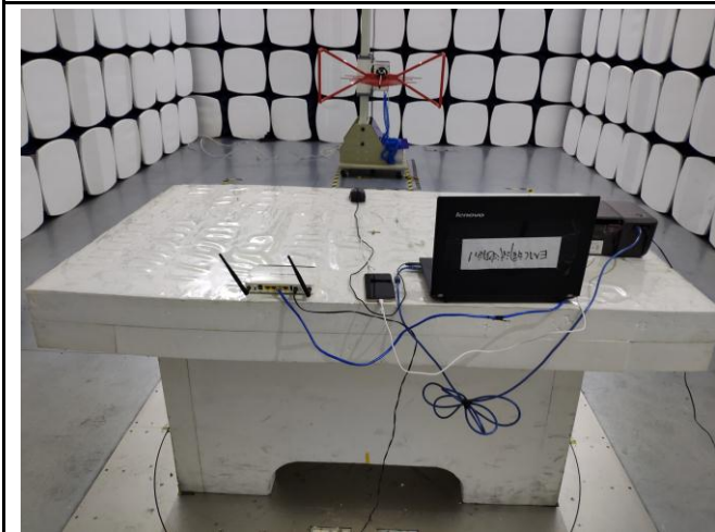
Radiated Emissions Test Setup Below 1GHz
