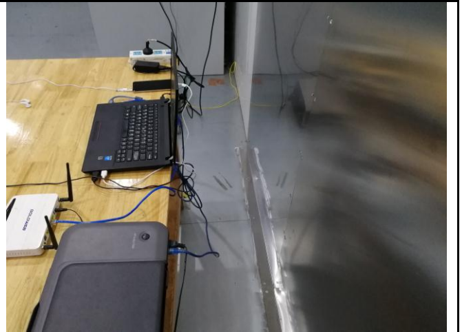
Conducted Emissions Test Setup – Side View
