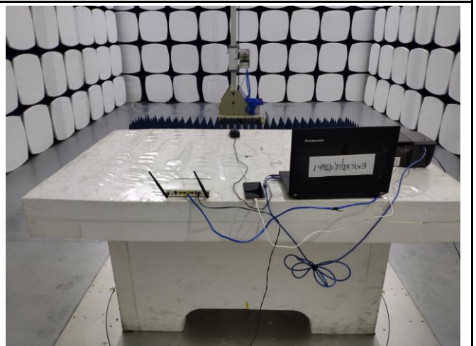
Radiated Emissions Test Setup Above 1GHz
