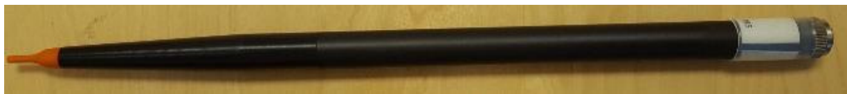
Figure 2 – MVG COMOSAR Dosimetric E field Dipole
